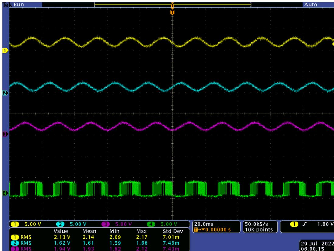
Figure 7.7. Profiles of phase A voltage of inverter-1 and inverter-2, current of inverter-1 and PWM signal for IGBT-1 of inverter-1 while controlled by SME-EDC before closing breaker-2 (before synchronism)
