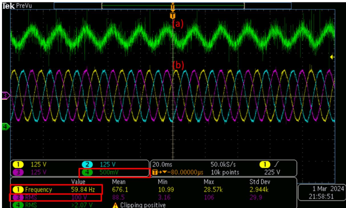
Figure. 7.16. Profiles of (a) inverter's scaled and shifted voltage ( $V_{mC}$ ) and (b) inverter's filtered output voltage ( $V_{PCC}$ ) while controlled by SME-EDC in closed loop control
