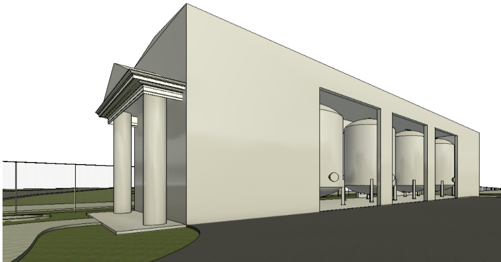
Figure 3.2.3.38: Low LOD Revit Model of GAC Building
