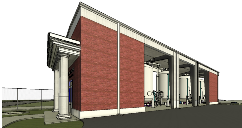
Figure 3.2.3.36: High LOD Revit model of GAC Building
