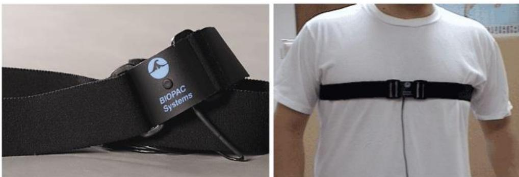
Figure 15: SS5LB transducer placement on Participant
