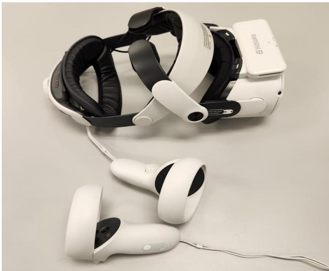
Figure 18: Meta Quest 2 with two additional features: a specialized head strap and a cooling fan.
