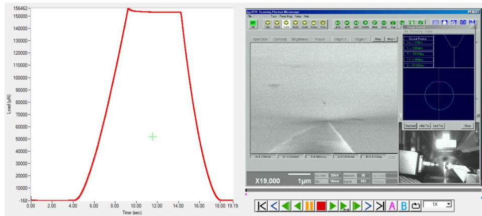
Figure 2.10 Screenshots of in-situ nanoindentation testing process performed on Si.
