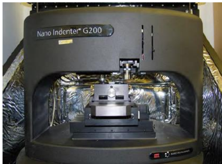
Figure 2.6 Photographs of Nano Indenter G200 (MTS).
