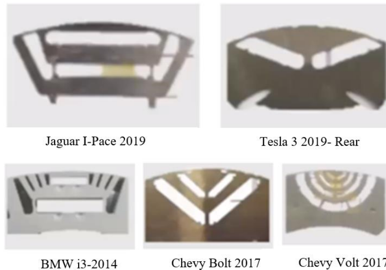
Figure 2.7. Design trend in air barrier type rotors of PM-SyRM [1].
