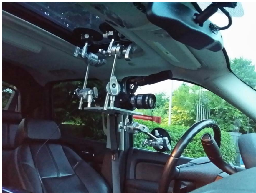
FIGURE 5: Sony NEX-FS100U camcorder mounted at a driver's height of eye
