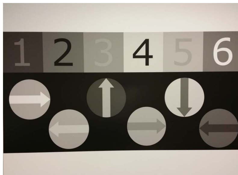
FIGURE 4: Contrast board used to calibrate nighttime video
