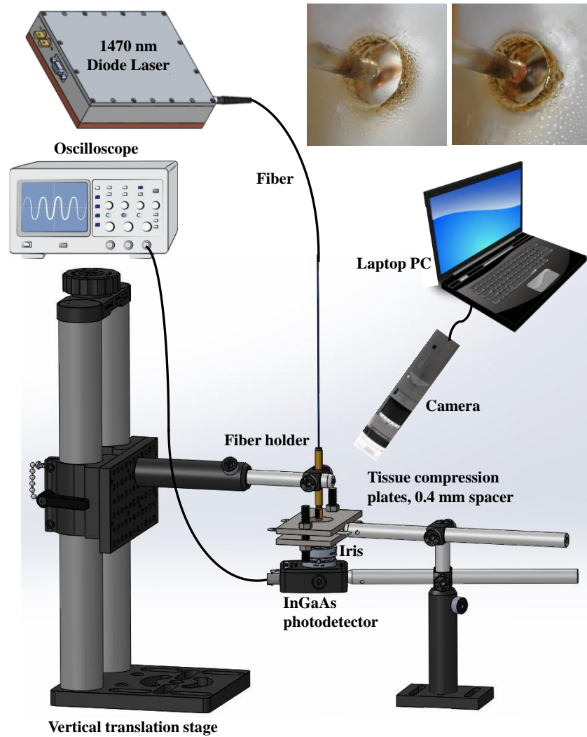
Figure 6.2: Experimental setup for acquiring the optical transmission signal during continuous-wave laser ablation of compressed porcine renal blood vessels. (Left top inset) Start of formation of a carbon layer on the tissue surface during laser irradiation. (Right top inset) Formation of a hollow crater during irradiation.
