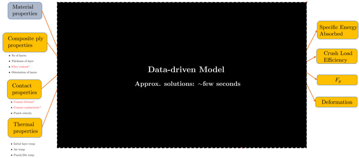
Figure 2.9: Simulation workflow replaced by black-box reduced order model
