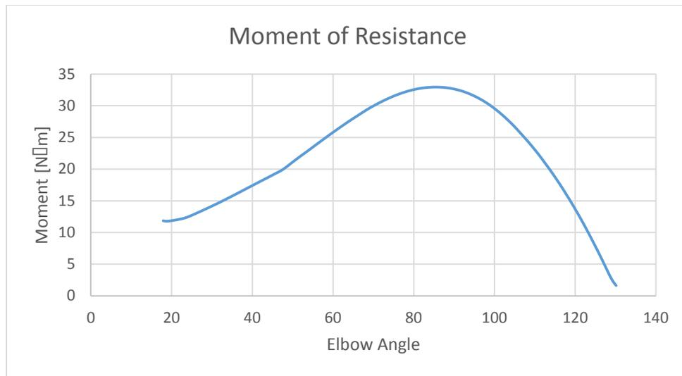
Figure 53: Moment of resistance curve for the Trial 3 (SB Floor) kinematic motion.
