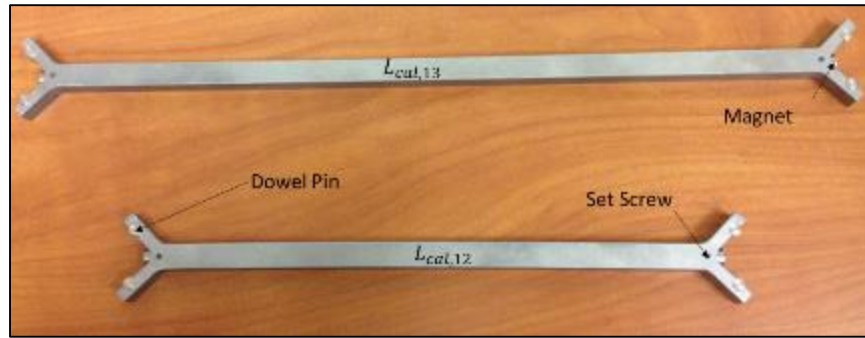
FIGURE 32: Reference length standards for identification routine, first design of measuring instrument
