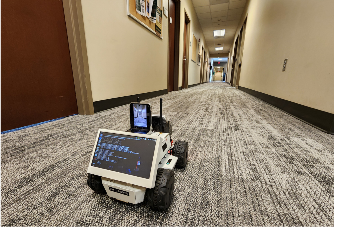
Figure 2.6: AgileX LIMO robot with camera mounted on top.
