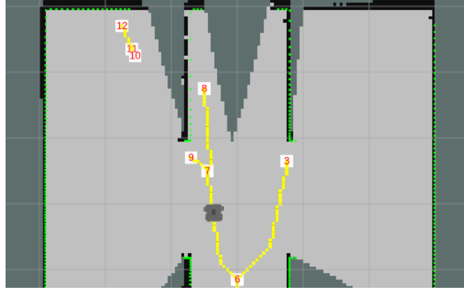
Figure 3.11: Robot exploring the Straight Corridor Gazebo environment, moving along an edge of the skeleton graph. Skeleton graphs in Gazebo environments generate multiple vertices along the direction from the robot’s current position to the exploration frontier. Here the vertices (7, 9, 8) are along the corridor. The skeleton graph shown here will be updated using the updated map after the robot reaches the target vertex. The frontier is the boundary between the light gray and dark gray regions of the map.
