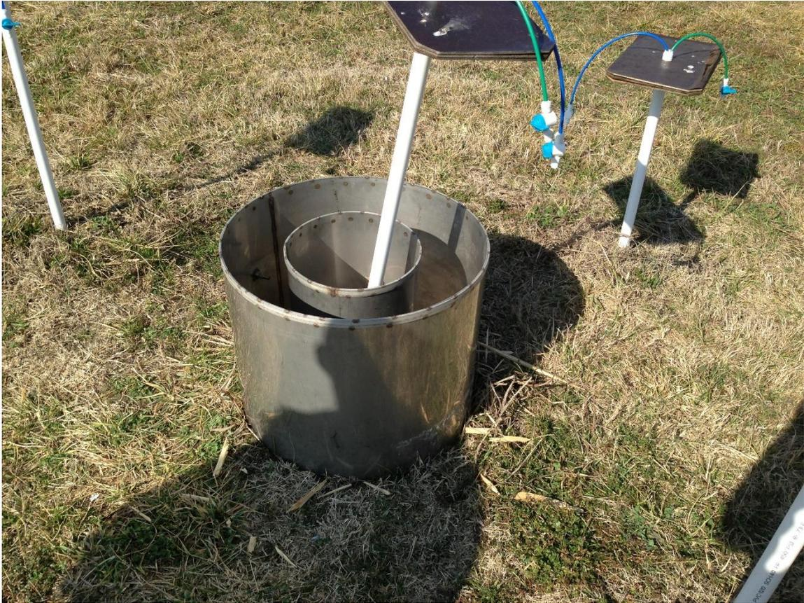
Figure 10: Double ring infiltrometer used for field attenuation study
