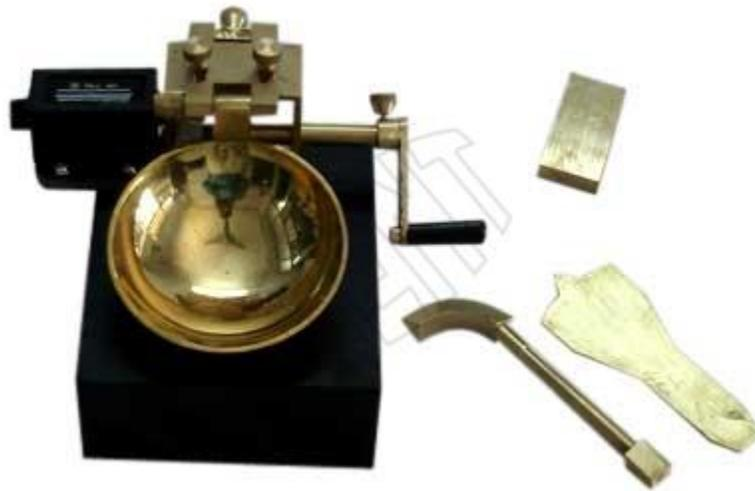
Figure 11: Casagrande apparatus
