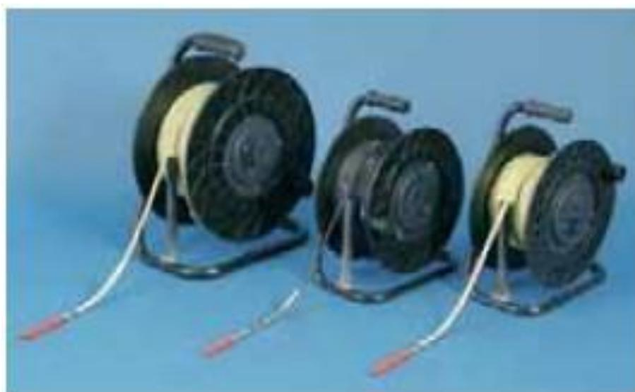
Figure 8: Water contact meters
