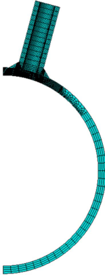
Figure 3.9: Final mesh for the IN740H model 15,232 C3D20RT elements.
