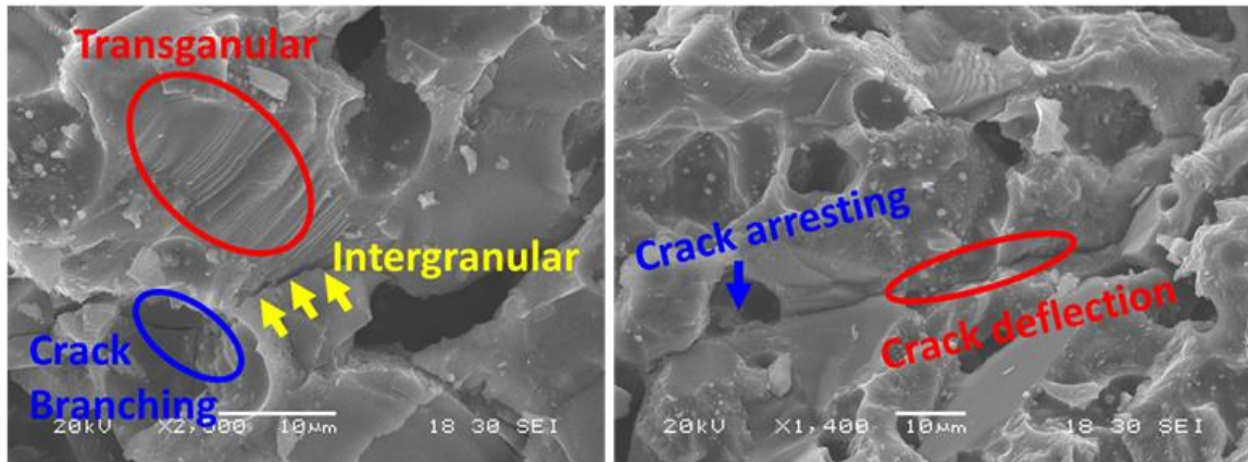
Figure 42: SEM examination of the fracture morphology in SiC-mullite (85SiC/15ash samples) heat treated at 1400 °C/1hr reveals various fracture characteristics observed on the sample's fracture surface [191].
