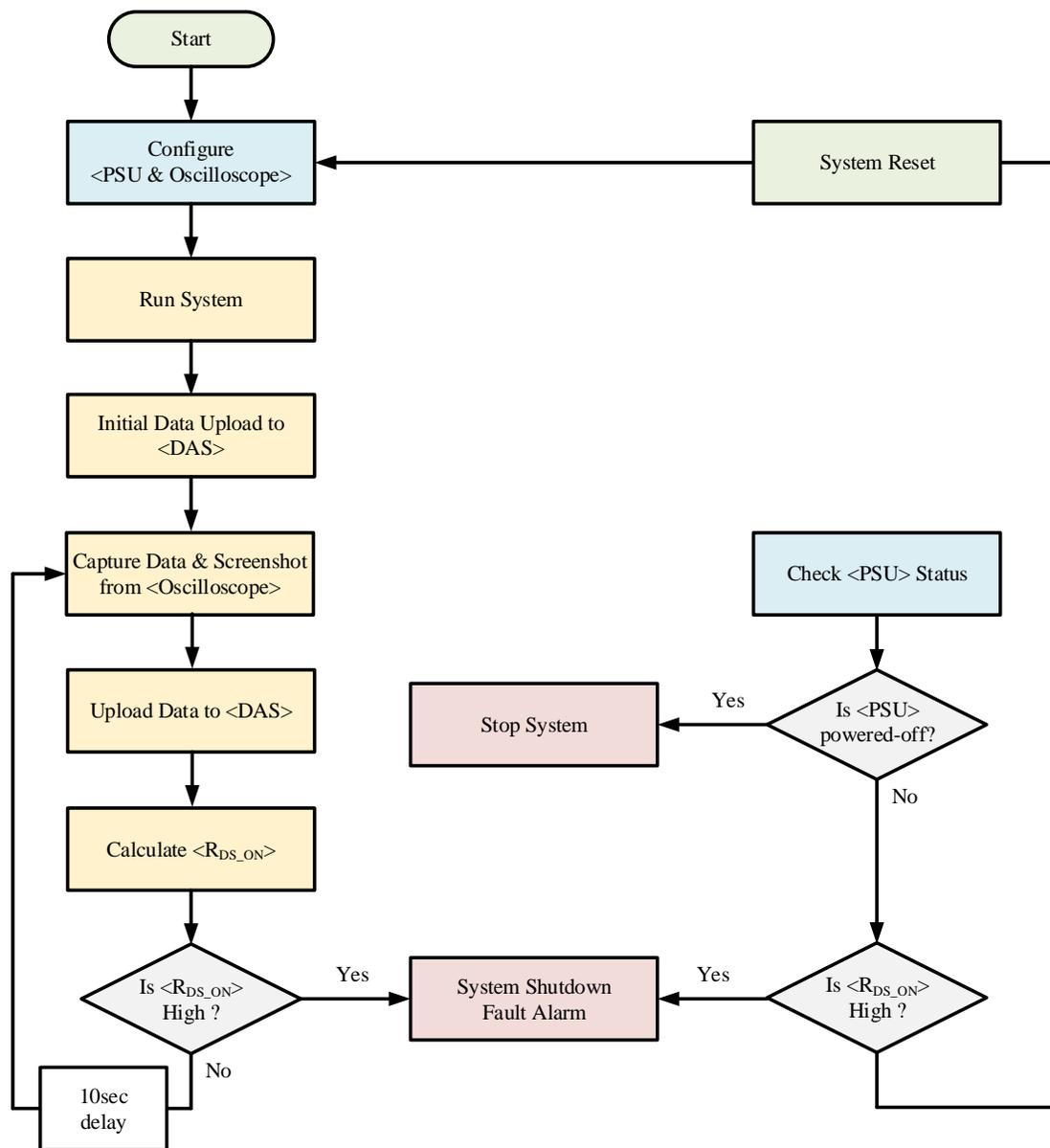
Figure 5.5: **Data acquisition system:** The thread is provided for device characterization and resistance measurement.
