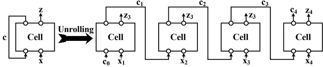
Figure 4.4: **Recurrent Neural Networks:** The schematic of standard RNN cell and its unrolling version for four input time sequence
