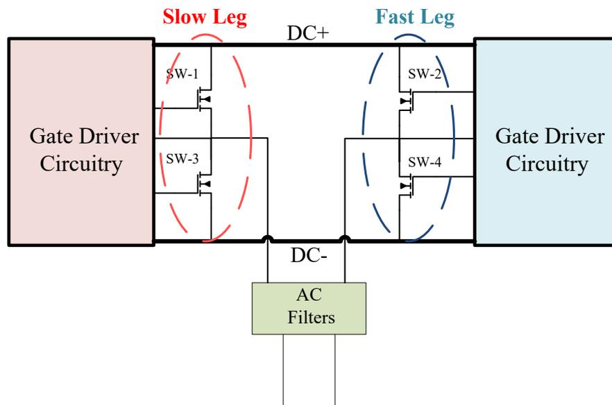
Figure A.1: **Schematic configuration:** The hybrid sinusoidal unipolar DC-AC converter topology considering one leg as fast switching, the second leg switching with grid frequency.
