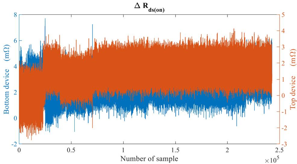
Figure 5.6: **The filtered on-resistance variations:** The 400W buck prototype was tested over 30G cycles with continuous operation at 100kHz switching frequency, and drain-source resistance variations was captured automatically.
