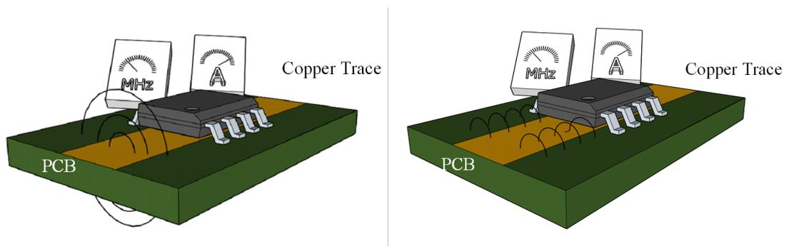
Figure B.4: **Magneto-Resistors sensor:** General operation of the contact-less AMR sensor: magnetic field generations at low frequency (left) and high-frequency (right) are shown.
