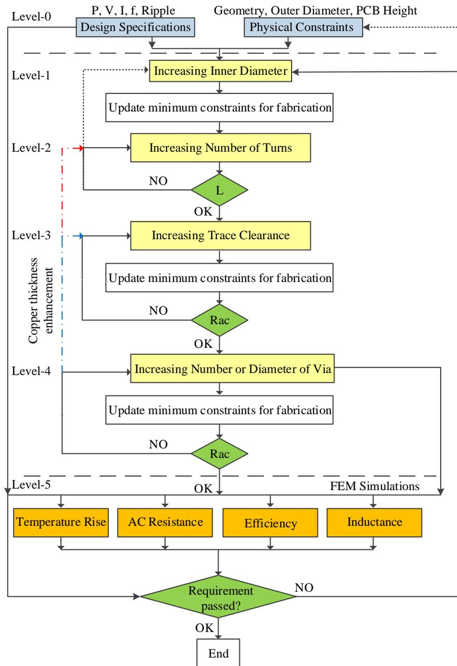
Figure A.2: **Optimization approach:** The algorithm descriptions to achieve the lowest resistance at the highest possible power density for the PCB embedded inductor within the 1-10MHz.
