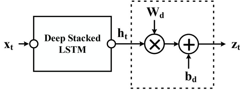
Figure 4.8: **The proposed deep LSTM network model:** A linear layer is added to the deep stacked LSTM to map  $h_t$  to on-line measured  $\Delta R$  at time  $t$ .
