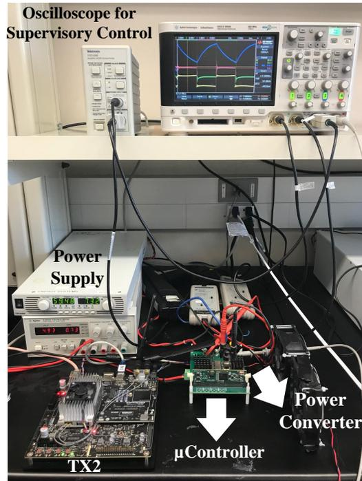
Figure 6.9: **Experimental verification:** The hardware setup was implemented including the high-frequency power converter controller by  $\mu$ -controller, the SoC-TX2 for edge computation. The supervisory control is designed for the safety protection.
