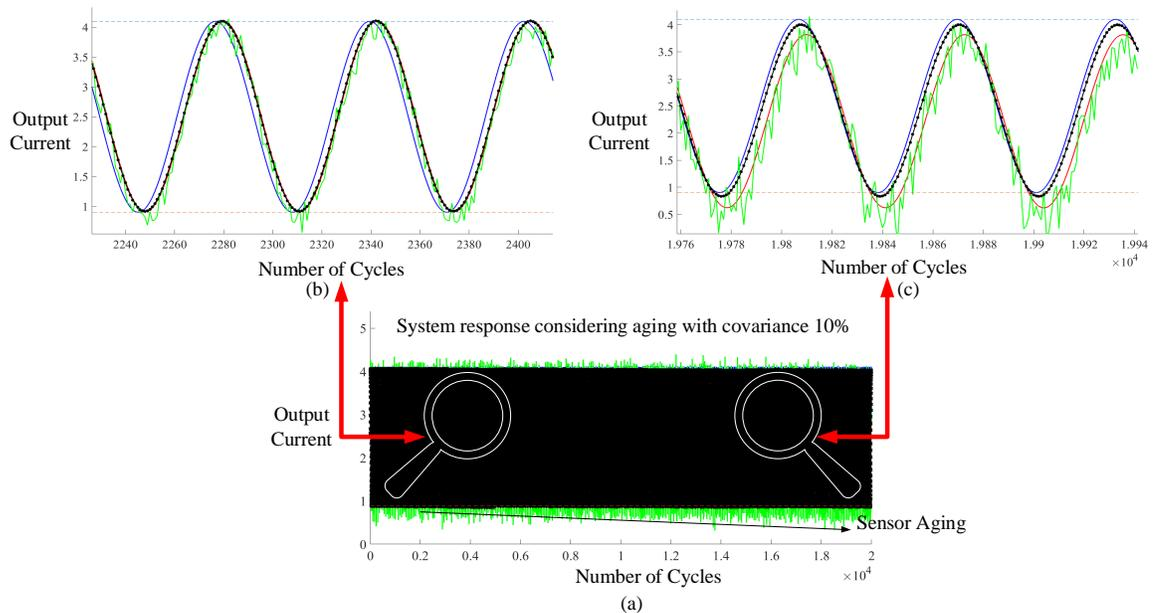
Figure C.5: **Simulation results:** The estimation results considered by a Kalman filter to the modified model of current sensor aging. The system response is modeled with 10% covariance error of the current sensor and shown based during the aging process. blue: ideal waveform, green: actual sensor measurement, red: system response correction with Kalman filter without aging considerations, black: system response correction with Kalman filter considering the aging process.
