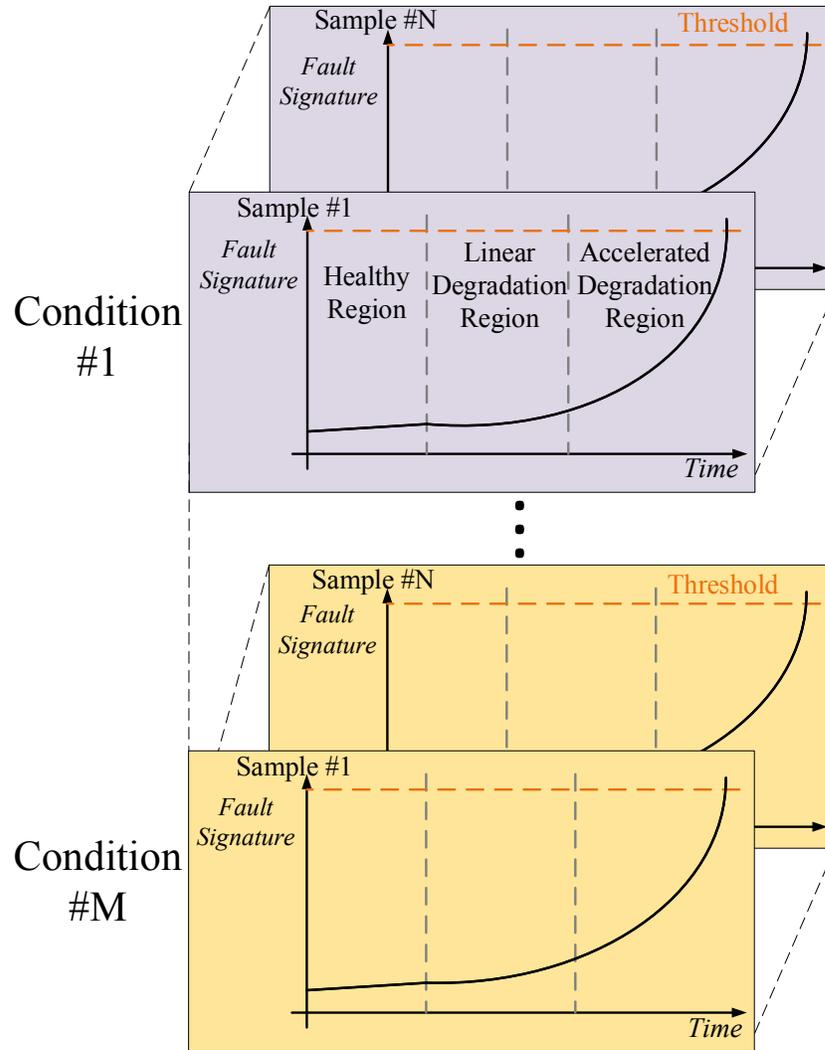
Figure 3.1: **Conventional reliability solution:**  $\#N$  samples of devices with  $\#M$  conditions have been analyzed experimentally under accelerated life tests to find the reliability model. Adaptability with the new technologies and the experimental costs are their main drawbacks.
