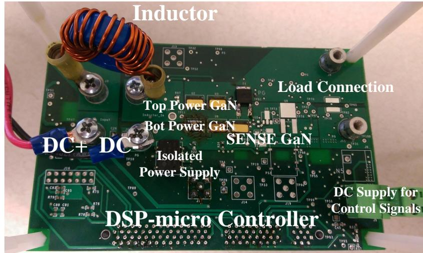
Figure 7.4: **Hardware setup:** The prototype was designed in four layers: Top layer: Power stage, Inner layer-1: Power ground, Inner layer-2: Shield layer, Bottom layer: Control signals and conditioning circuits.
