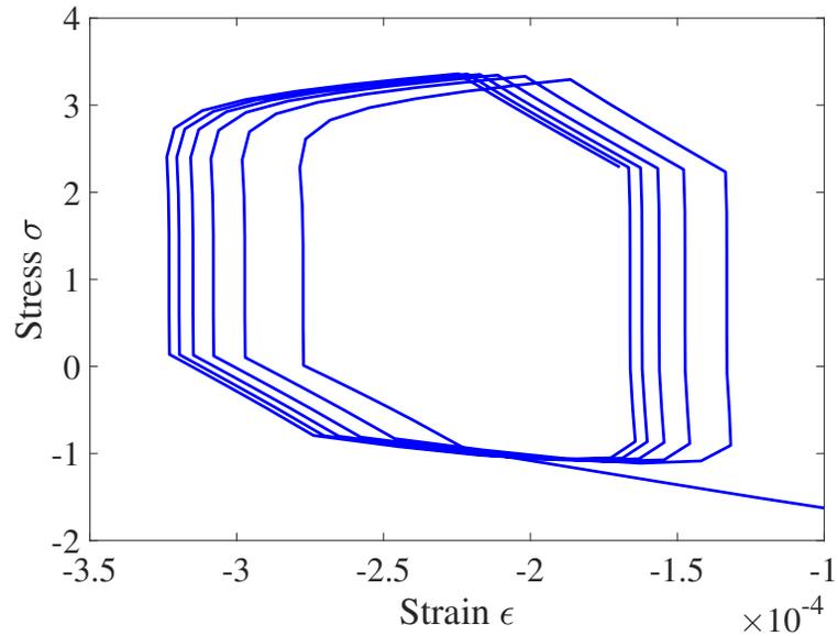
Figure 3.8: **Simulation of strain-resistance:** The simulated energy loss generated from the stress and strain variation of the joints in the accelerated life analysis.
