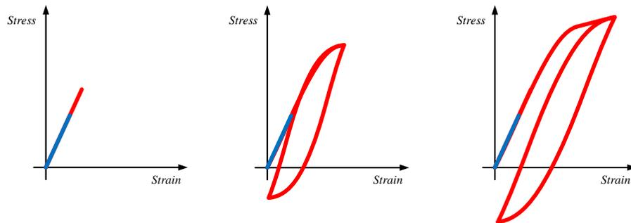
Figure 3.4: **The hysteresis loss:** Once the nominal mean stress is less than border mean stress (left) vs. the mean stress is higher than the border mean stress (right).
