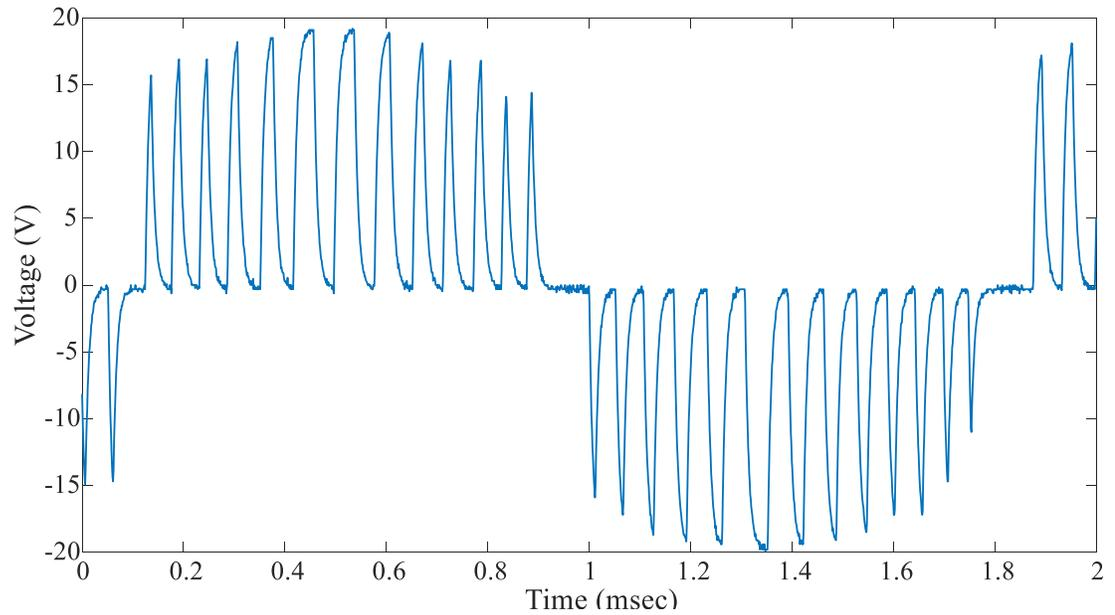
Figure 7.23: **SenseGaN for the BCM control of a DC-AC converter:** Two reference trigger signals are considered to turn-on the bottom devices consecutively. The closed loop operation of the DC-AC converter operation is verified in CHIL (blue: grid voltage)
