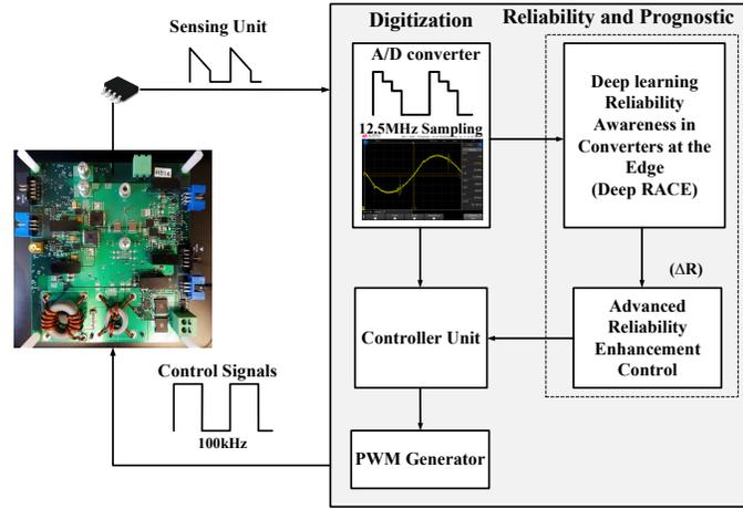
Figure 5.1: **The edge node diagram:** It consists of a  $\mu$ -controller and AI SoC to generate gate signals and predict the trajectory resistance of power transistor.
