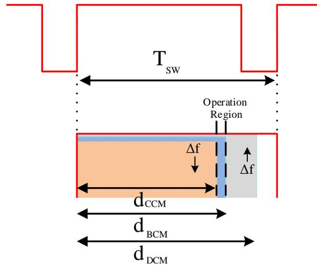
Figure 7.8: **The system operation modes:** The operational regions for distinguishing CCM, BCM, and DCM in a single cycle. Orange: CCM, Blue: Optimum region for BCM, Gray: DCM.
