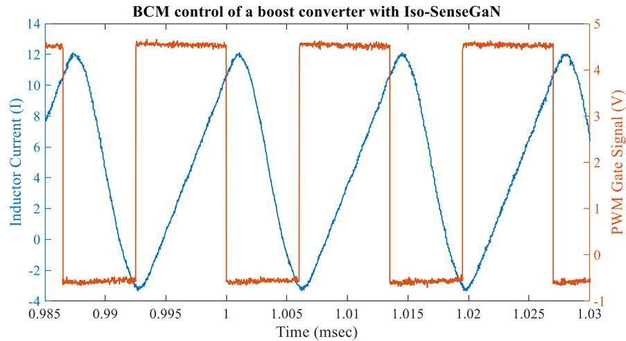
Figure 7.18: **BCM control of a DC-DC boost converter:** orange: PWM gate signals, blue: inductor current.
