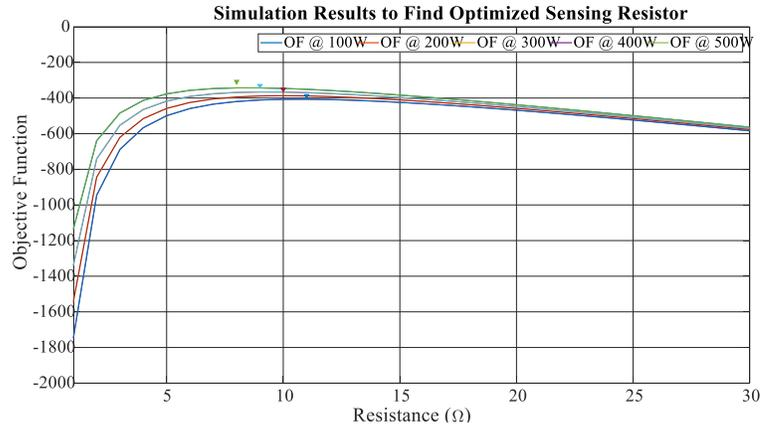
Figure 7.15: **Optimization in SenseGaN**: The compromise of higher performance (low resistance) vs. lower loss (high resistance) are analyzed in the OF.
