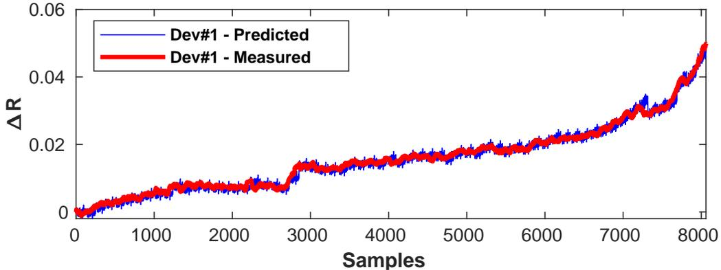
Figure 6.2: **Experimental results:** The prediction of  $\Delta R_{ds(on)}$  variations of device-1 through Deep RACE method.
