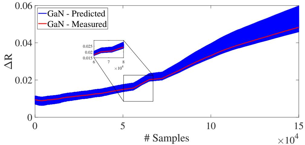
Figure 6.11: **Prognostic results:** The  $R_{ds(on)}$  variations for GaN with Si-substrate using the FEA simulations, and only one set of data for training.
