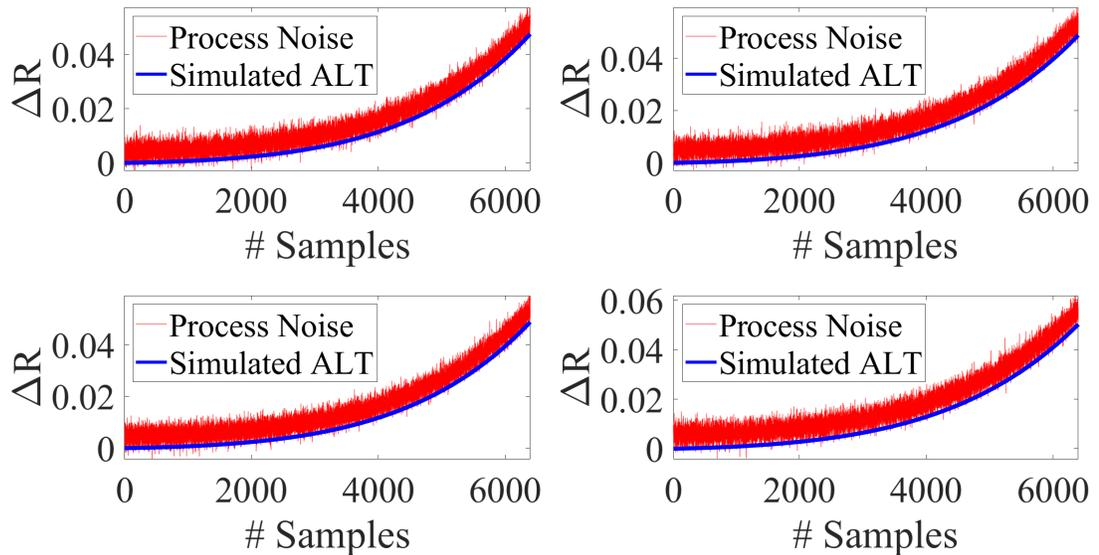
Figure 3.9: **Simulation result of the accelerated life test:** The variations  $R_{ds(on)}$  under temperature cycling due to solder fatigue of GaN on Silicon.
