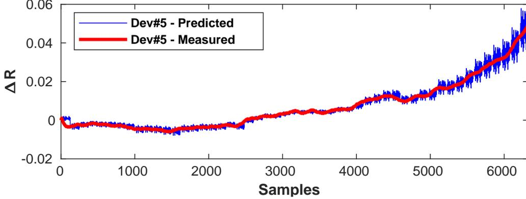
Figure 6.6: **Experimental results:** The prediction of  $\Delta R_{ds(on)}$  variations of device-5 through Deep RACE method.
