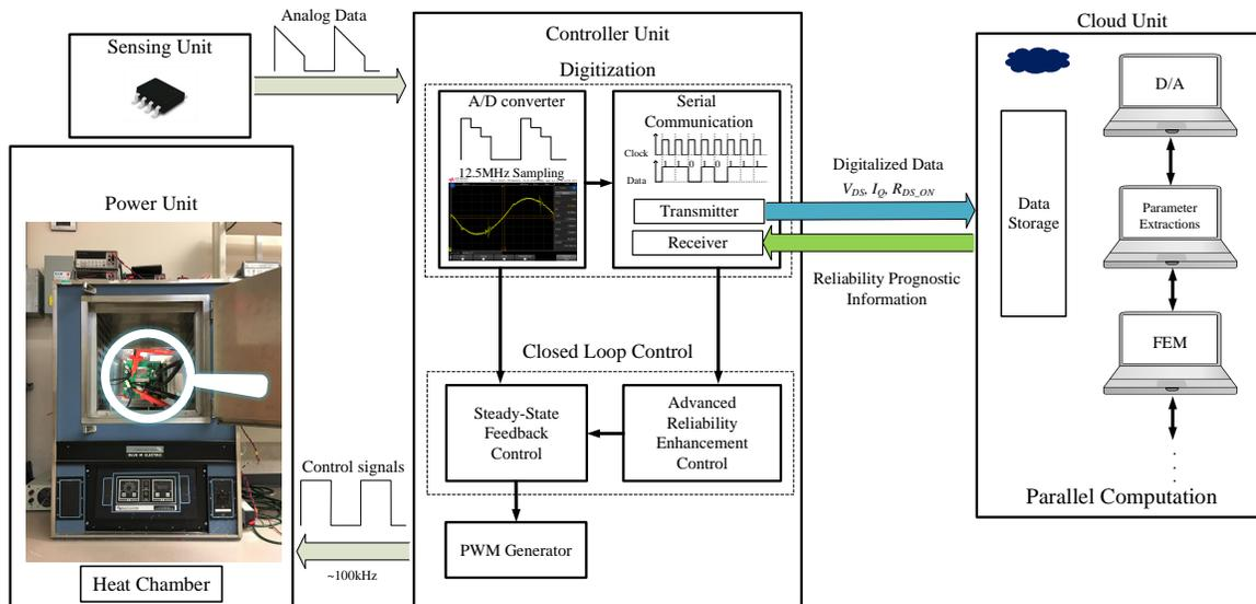
Figure 5.2: **New IoT approach for reliability assessment:** DAS for characterization of power converters, and multi-process computation on cloud networks. The proposed infrastructure architecture provides feasibility of data-processing techniques for adaptive prognostics in power electronics converters.
