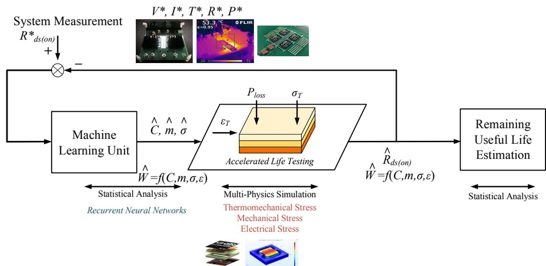
Figure 3.5: **Proposed framework for GaN power converter-Digital Twin:** The online device monitoring, and simulation-based ALT for reliability analysis. A machine learning system is developed for system calibrations and parameter estimations.
