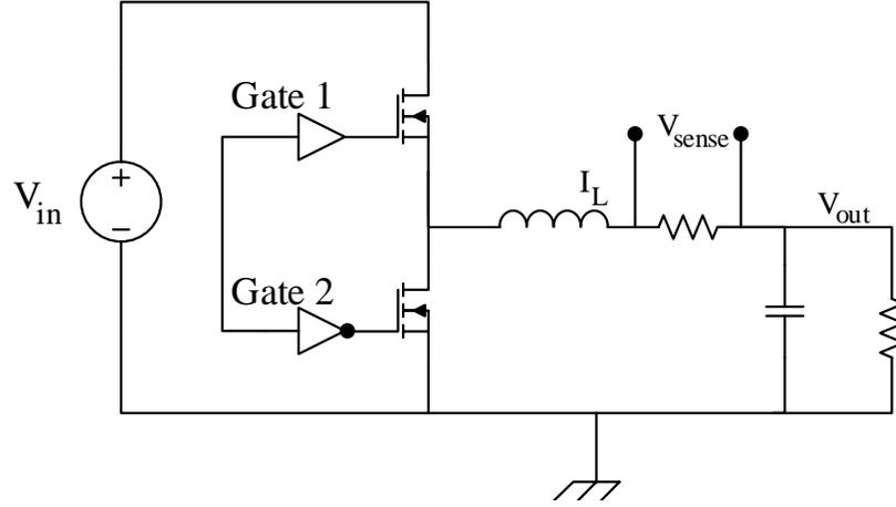
Figure B.1: **Shunt method**: Schematic of external sense resistor for capturing the inductor and output current. The voltage drop across the resistor theoretically can represent the actual current waveform; however, this method in practice has a lot of issues for high-frequency and high current applications.
