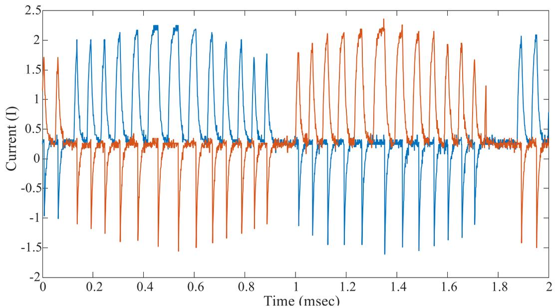
Figure 7.24: **SenseGaN for the BCM control of a DC-AC converter:** Two reference trigger signals are considered to turn-on the bottom devices consecutively. The closed loop operation of the DC-AC converter operation is verified in CHIL (top: bottom SenseGaN-1, orange: bottom SenseGaN-2)
