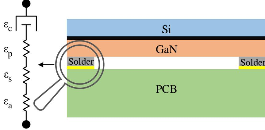
Figure 3.3: **Mounted GaN on the PCB:** Simplified model of a lateral GaN mounted on the PCB. GaN and Silicon (substrates) are isolated with thin layer of AlGaN, and packaging is not considered in the model.
