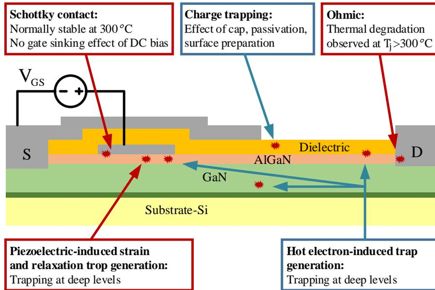
Figure 2.2: **Lateral GaN structure:** The most susceptible regions in GaN device.
