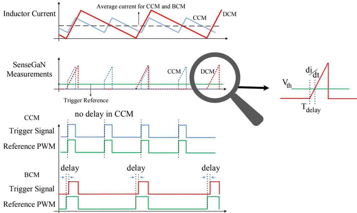
Figure 7.7: **The system operation mode and cursor identifications:** a) The inductor current at CCM (blue) and BCM (red) with the same average current. b) The current monitoring with the SenseGaN for the active device in CCM and BCM. (here, the zoomed-in version of threshold trigger reference signal for delay generation is exposed) c) The microcontroller compares the trigger reference signal generated by the comparator and PWM signals to generate the delay signal in CCM and BCM.
