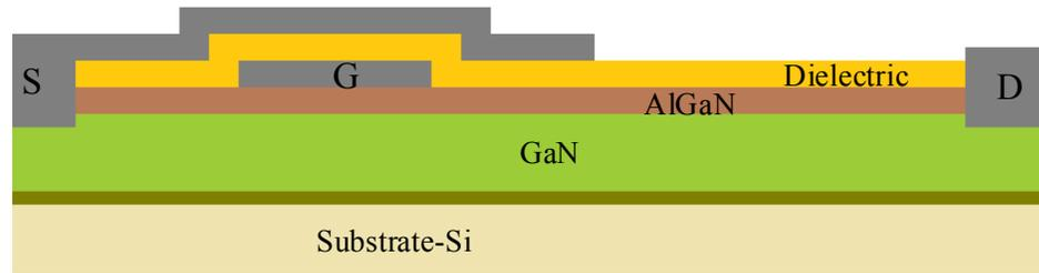
Figure 2.1: **Lateral GaN structure:** The cross section of an enhancement GaN.
