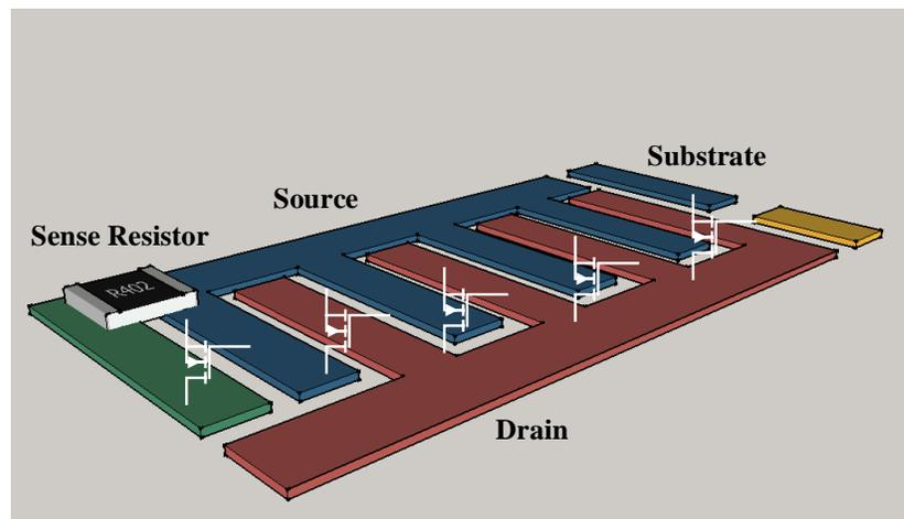
Figure 7.12: **Iso-SenseGaN configuration:** Proposing a scheme of Iso-SenseGaN for lateral dies based on available commercial products.
