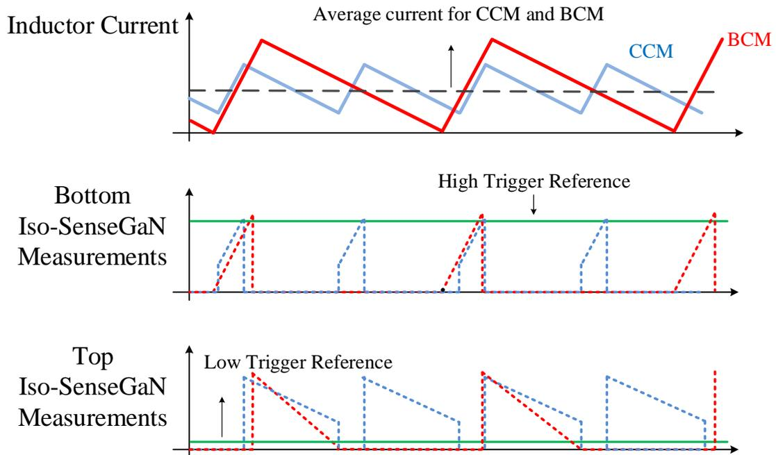
Figure 7.17: **BCM control of a DC-DC boost converter:** the current monitoring reflected in the Iso-SenseGaN. Two reference trigger signals are considered to turn-on the top and bottom devices consecutive.
