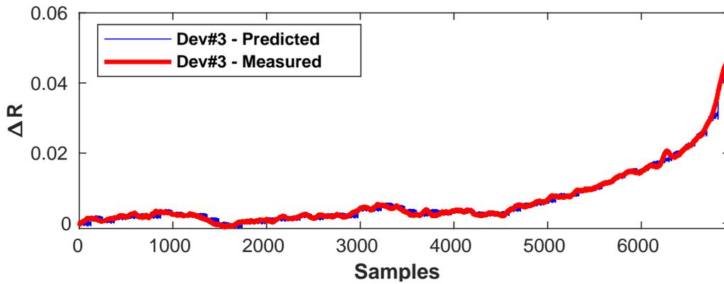
Figure 6.4: **Experimental results:** The prediction of  $\Delta R_{ds(on)}$  variations of device-3 through Deep RACE method.
