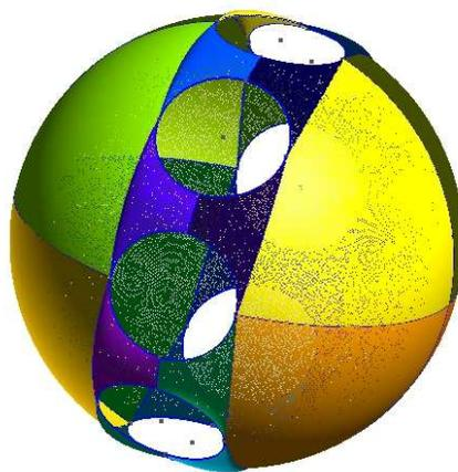
Figure 19: Boundary mesh generated by GMSH on off-electrode patch.
