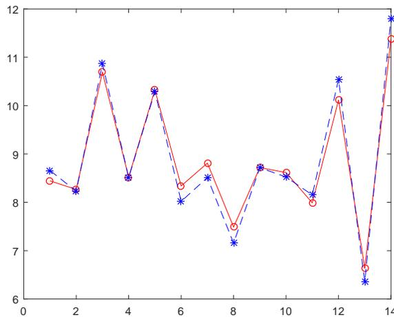
Figure 15: Exterior Neumann problem for the domain in Fig.13: exact potentials (asterisks) and numerical solutions (circles) on the boundary with a relative error of 2.31%.  $\Delta x = 5 \times 10^{-4}$ ,  $\varepsilon = 3\Delta x$ ,  $N=2 \times 10^4$ ,  $NT = 5 \times 10^4$ .
