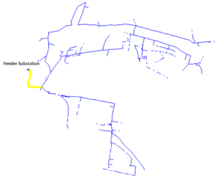
Figure 3.5: CyME model of the overloaded feeder F2
