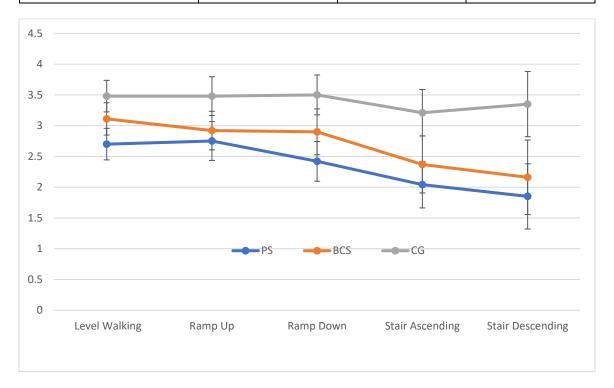
Figure 5.17 Knee Biomechanical Index (Mean  $\pm$  Standard Deviation) in Five Daily Activities for Posterior Stabilized Implant, Bi-cruciate Stabilized Implant, and CG.
