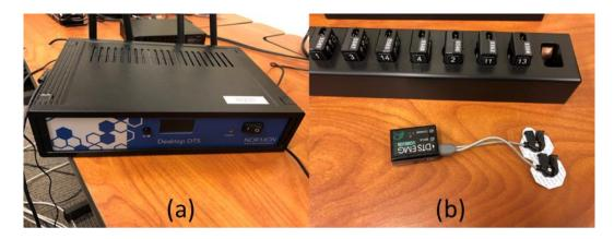
Figure 4.11 Noraxon EMG System. ((a): The Desktop DTS EMG Receiver (b): The EMG Transmitter and Electrodes)
