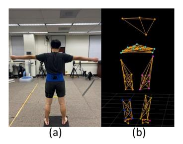
Figure 2.7 (a) T-pose and (b) Digitized Model.
