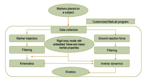
Figure 4.7 MATLAB Flow Chart for Motion Data Analysis.
