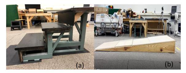
Figure 4.2 (a) Customized Stairs (18cm Height, 70cm Wide) and (b) Ramps (3m Long, 1m Wide, 15 Degrees) in Motion Lab.
