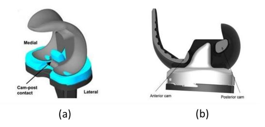
Figure 2.5 (a) Posterior Stabilized TKA Implants and(B) Bi-cruciate Stabilized TKA Implants [3, 32].
