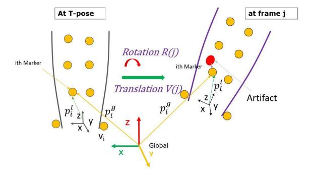
Figure 4.8 Tracking Motion of Rigid Body.
