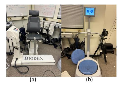
Figure 2.9 (a) Biodex Dynamometer and (b) Biodex Balance System.
