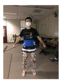
Figure 2.6 Marker Set Used and High-speed Cameras of a Motion Capture System.
