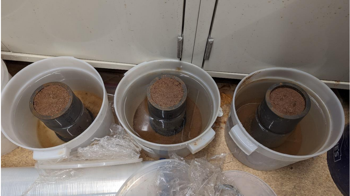
Figure 8-4 Compacted samples soaked in buckets.
