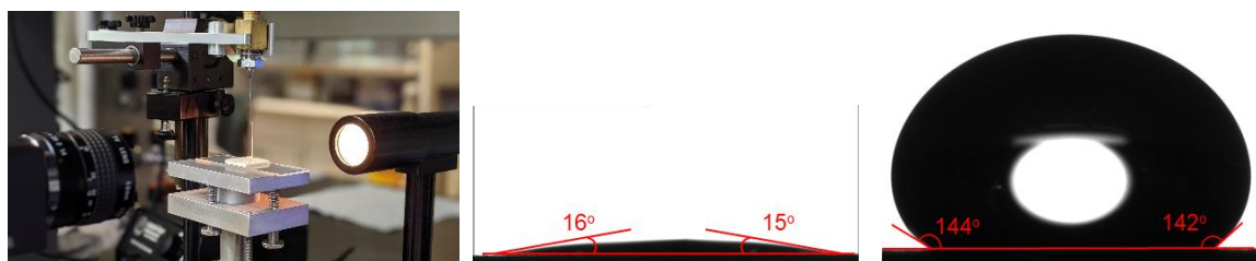
Figure 1-2 (a) Contact Angle measurement (b) Hydrophilic (<90°) (c) Hydrophobic (>90°)
