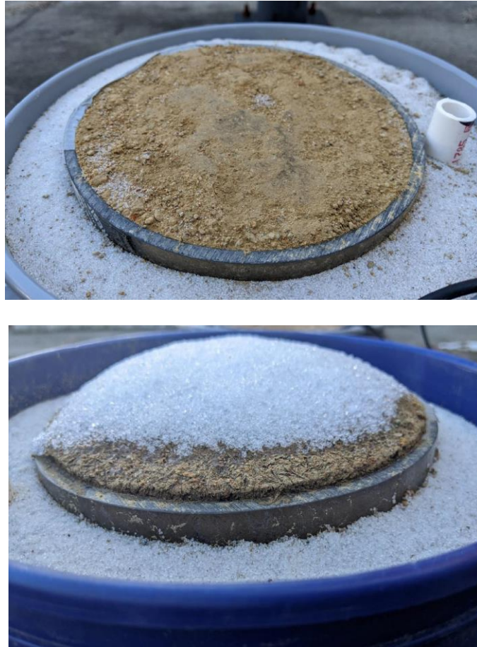
Figure 7-6 a) Water beading on treated sample b) Treated sample without heave, d) Untreated sample showing heave (~6mm)(Uduebor et al, 2023)
