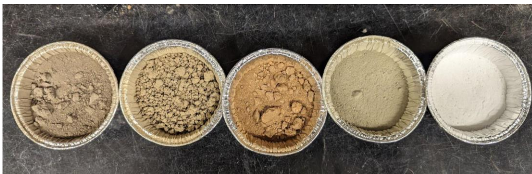
Figure 2-2 Soils and Glass Beads Utilized in this Study; AK-FB, IA-PC, NC-BO, NH-HS, and GB (Uduebor et al., 2023)
