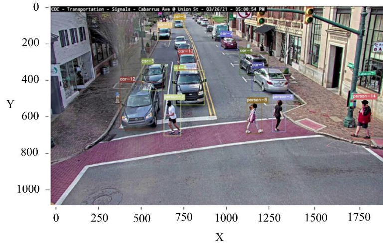
Figure 9. Illustration of detected and tracked pedestrians and vehicles at the fixed-cycle intersection
