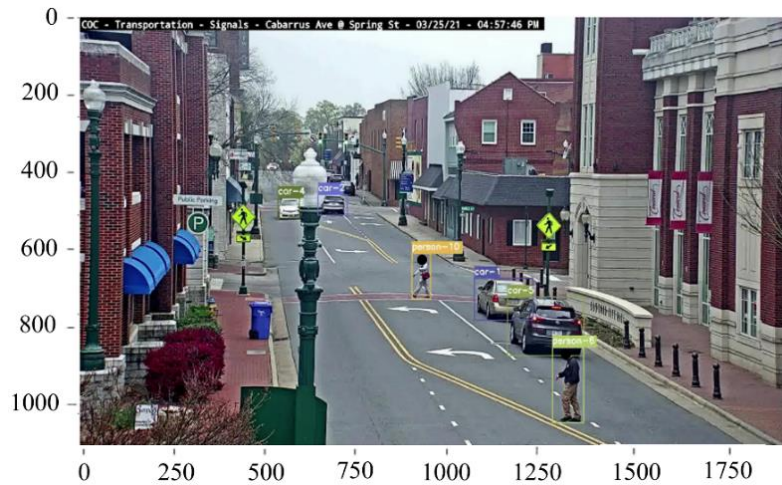
Figure 19. Illustration of detected and tracked pedestrians and vehicles at the RRFB-controlled intersection
