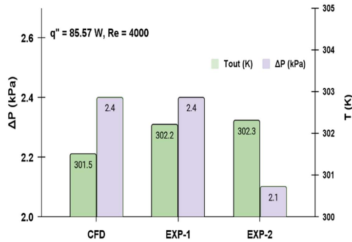
Fig.25 Results for constant heat input (Re=4000).
