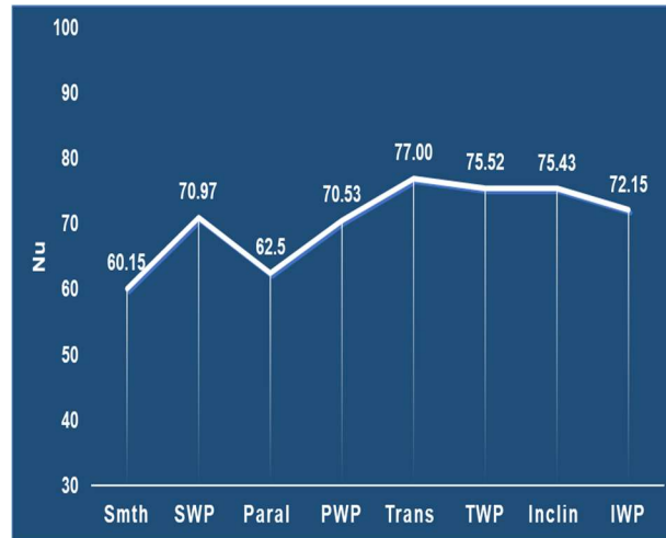
Fig. 5 Nu for turbulent flow ( Re = 4000 ) conditions. See the nomenclature section for interpretation of the horizontal axis labels.
