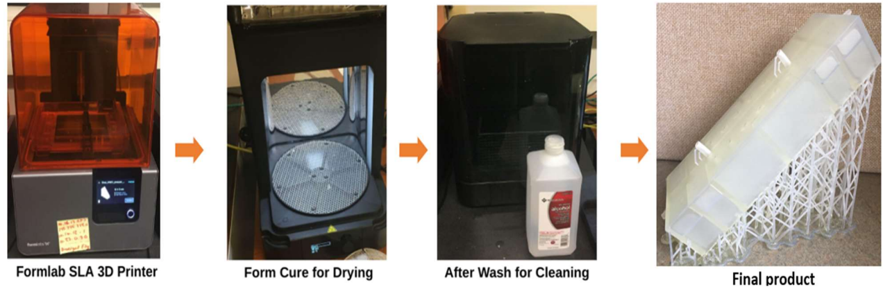
Fig. 2 3-D printing of resin part through SLA technique.
