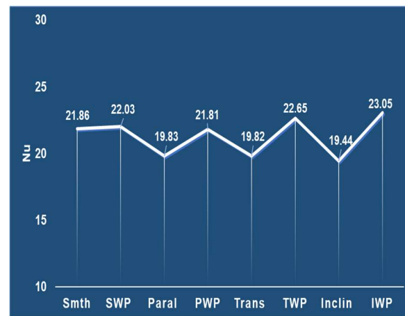
Fig. 6 Nu for laminar flow ( Re = 1000 ) conditions. See the nomenclature section for interpretation of the horizontal axis labels.
