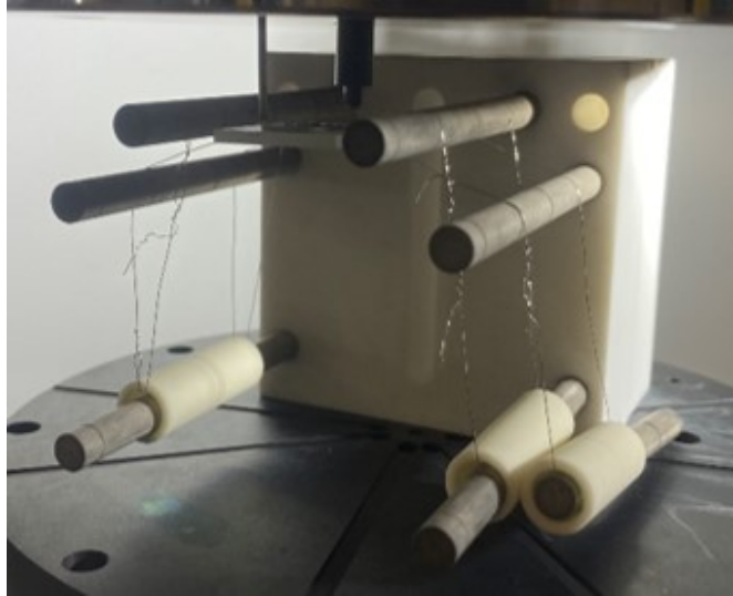
Figure 4.2: Glass sample suspended at the two nodes of their first vibration mode.
