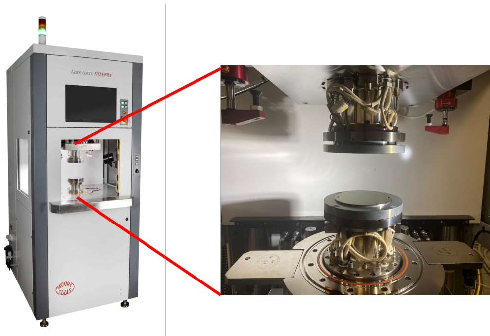
Figure 3.2: Precision glass molding machine (Moore Nanotech GPM170).
