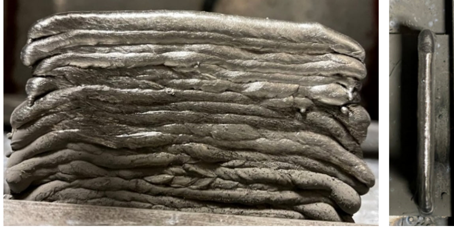
Figure 3.18: Stacked layers of low-IER printed wall during the deposition process (left) and bead profile from the top view (right).
