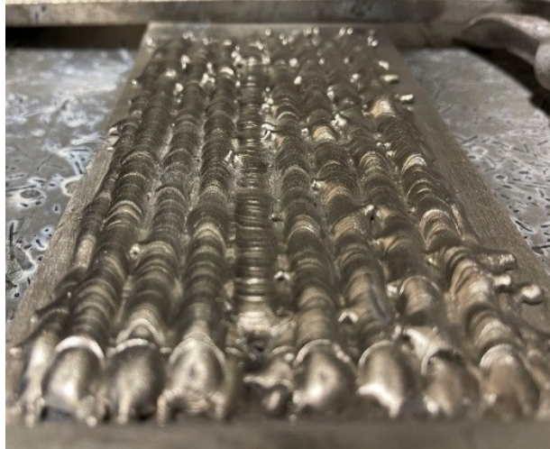
Figure 3.35: Long bead base layer deposition with channels resulting in a 50% overlap.
