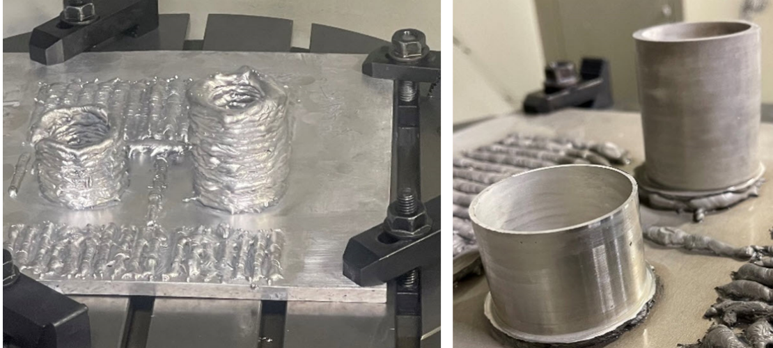
Figure 5.8: AZ31b Substrate with high and low-IER printed AZ61a cylinders fastened in the Mori Seiki ready for outer layer removal (left) and finished machined parts (right).
