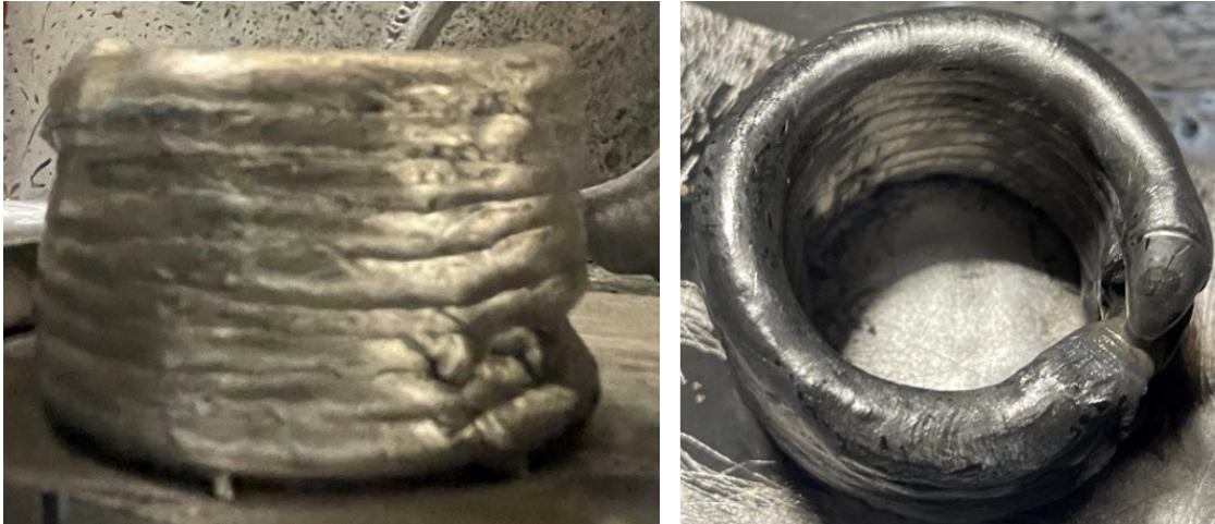
Figure 3.26: Layer fusion and shape retention during low-IER cylinder print (left) and closure problem evolution as layers are added to the printed part (right).
