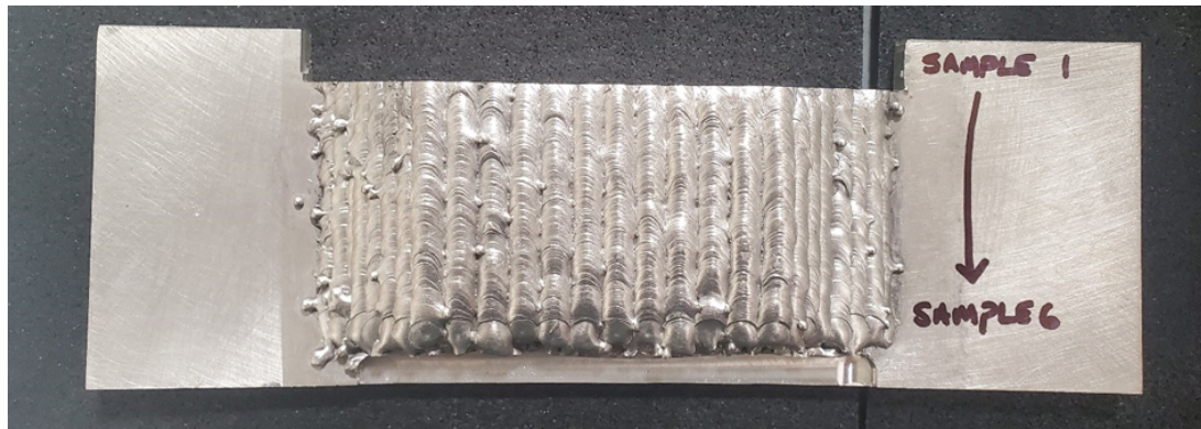
Figure 3.37: MRML block printed using staggered short beads to be used for tensile test specimen extraction and microstructure analysis.
