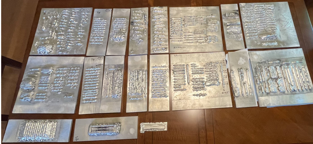
Figure 4.4: Initial TTS tests performed on CNC to determine the correct deposition parameters for high and low-IER magnesium deposition.
