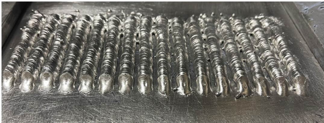
Figure 3.36: Short bead base layer channel deposition which will result in a 40% overlap.
