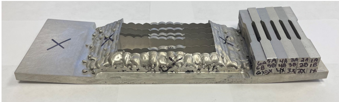
Figure 5.6: Example of wEDM tensile test coupon extraction from large WAAM printed magnesium blocks.
