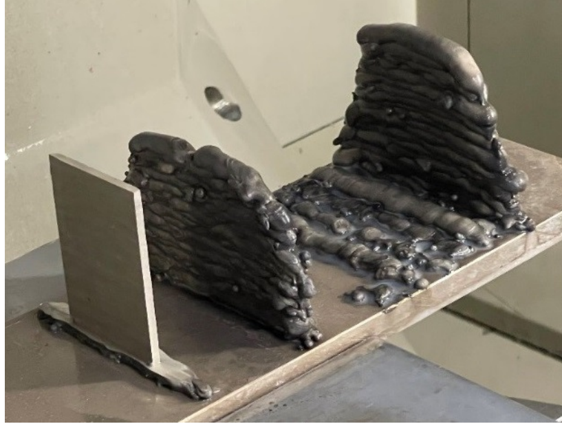
Figure 3.24: AZ31b substrate with AZ61a printed multilayer walls prepared for thin-walled machining.
