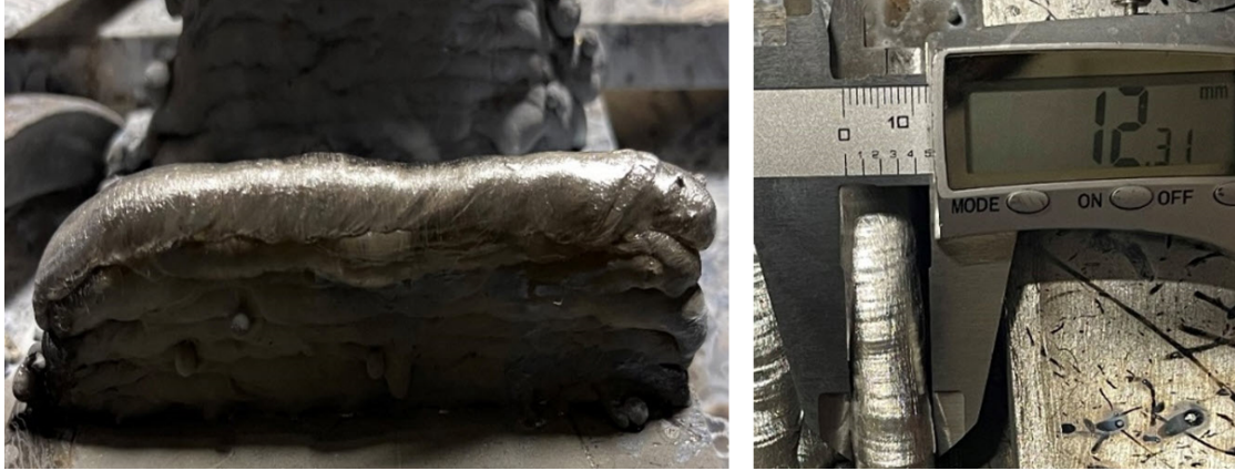
Figure 3.22: Bead profile of walls being deposited with high-IER (left) and width measurement of the beads as the layers were added (right).
