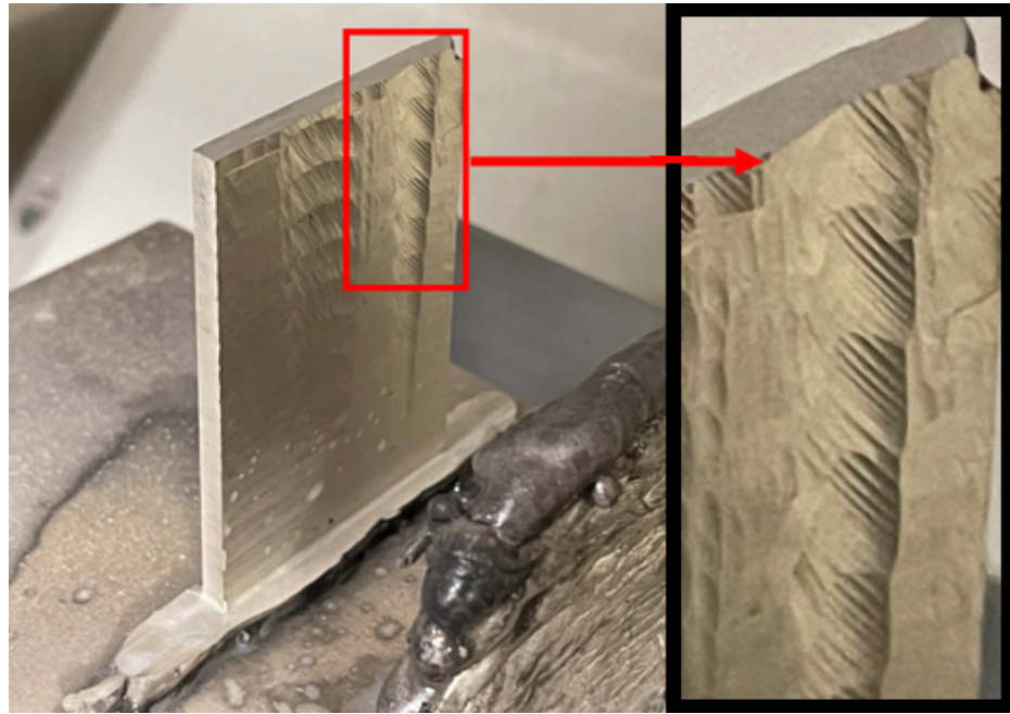
Figure 5.2: Severe chatter marks caused by insufficient depth of cut during thin wall machining of AZ61a.
