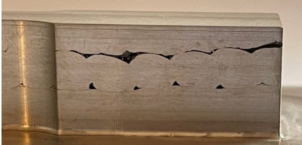
Figure 3.12: Lack of fusion between deposited magnesium layers caused by insufficient heat input.
