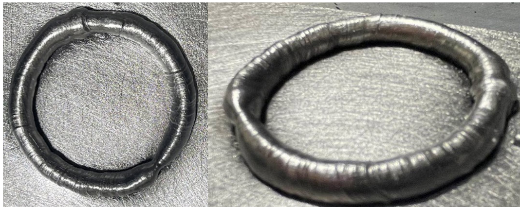
Figure 3.25: First layers of low heat input hollow cylinder print.
