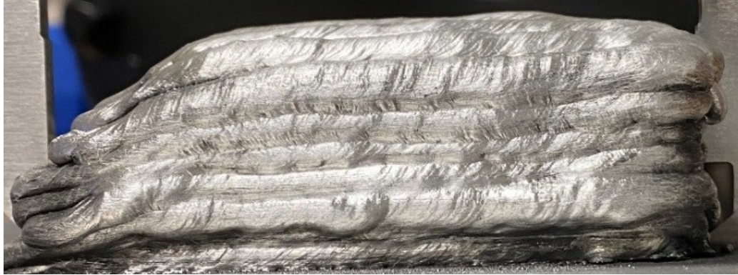
Figure 3.17: Gradual deterioration of multilayer block profile at the end point of bead deposition.
