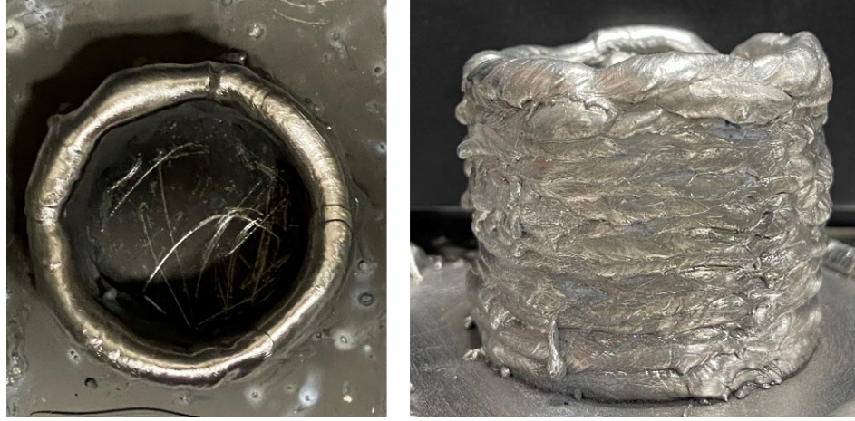
Figure 3.29: First two layers of printed cylinder with low-IER input parameters (left) and final printed hollow cylinder printed with low-IER with the top layer indicating pushback occurring during the deposition (right).
