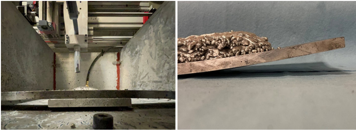
Figure 3.13: Severe substrate distortion inside the holding clamps of the CNC during the deposition of a large magnesium block (left), and final distortion of the substrate after having been removed from machine (right).
