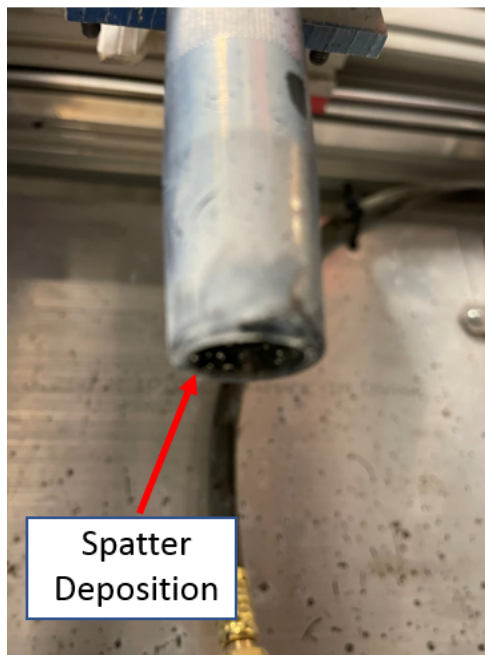
Figure 4.2: Spatter deposition inside the weld nozzle when the nozzle to workpiece offset distance is too small.
