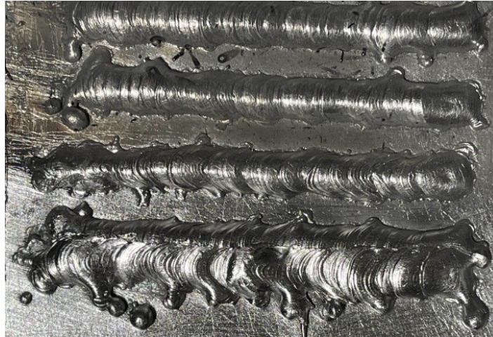
Figure 3.11: Example of how the low viscosity of melted magnesium causes severe side flow out of the weld pool during the deposition of overlapping beads.
