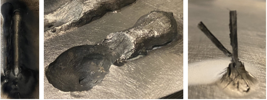
Figure 3.14: Magnesium oxide vapor layer around the AZ61a weld bead after deposition (left), top view crater left behind in substrate after AZ31b substrate ignited due to insufficient interpass cooling time and excessive heat input (middle), and bottom of substrate view at the crater location where molten magnesium flowed through the base (right).
