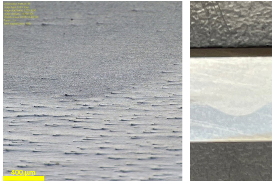
Figure 5.25: Interface between AZ31b substrate and AZ61a weld wire after etching with 2% Nital solution (left) and after polishing (right).
