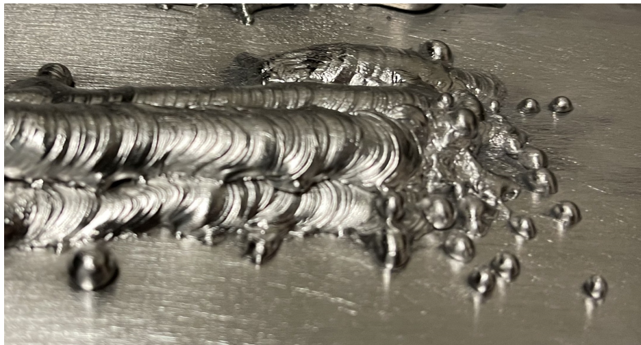
Figure E.2: DC spatter at very high-IER parameters.
