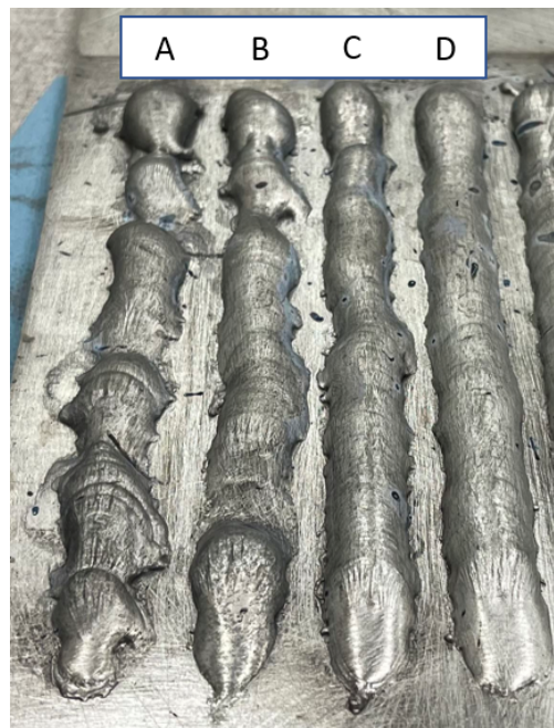
Figure 4.3: Improved bead continuity as TTS is decreased in increments of 50 mm/min from bead A to bead D while providing the same IER.
