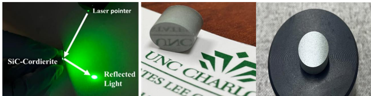
FIGURE 4.5 (left to right): Reflectivity experiment using green laser light on the polished surface of SiC-Cord; Reflection of the letters UNC; Surface of SiC-Spod disc polished to mirror finish.
