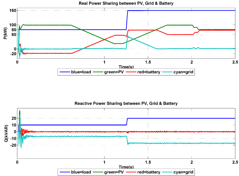
(c) Active and reactive power sharing in grid connected mode (load demand doubled at 1.25 sec)
