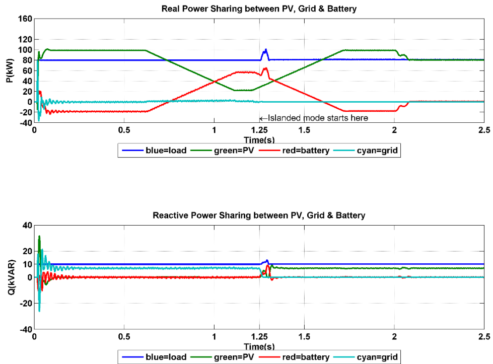
Figure 2-7: Active and reactive power sharing in islanded mode (Q supply from PV)
