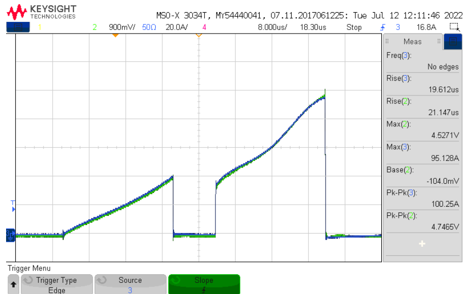
Figure 3.11: Double pulse test result, with equal pulse width of 50\mu s and duty cycle of %85. Blue is the proposed sensor output. Green is a reference 50A/50MHz current probe.
