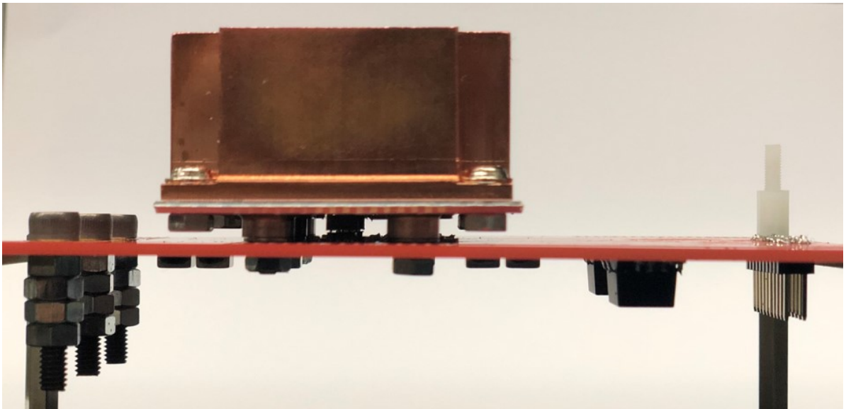
Figure A.8: Side-view of the connections made between the module and gate-driver.
