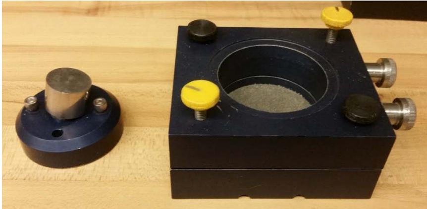
Figure 5.4: Direct shear box
