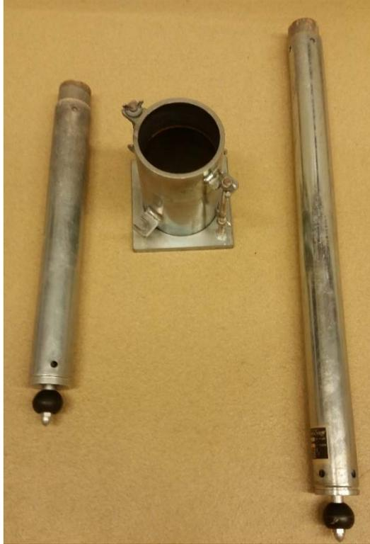
Figure 5.1: Proctor mold with standard and modified proctor hammers
