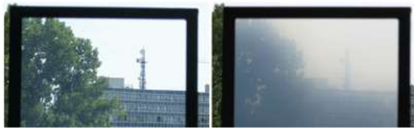
Figure 8: Effect of temperature on the thermochromic glass[23]
