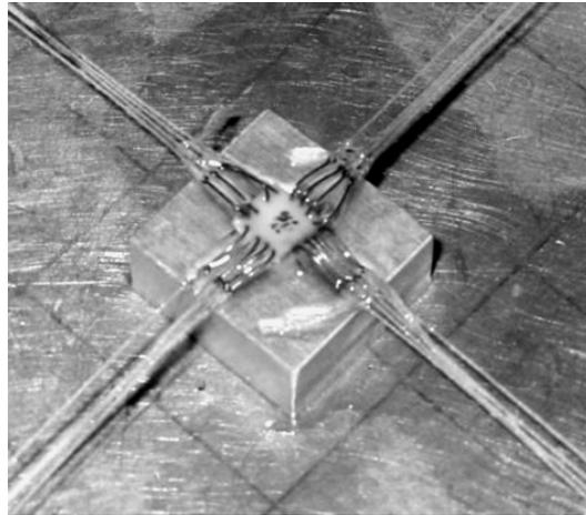
Figure 4: A square aortic section, mounted on four linear arms of a biaxial testing unit. Adapted from Lally et al. 2004.
