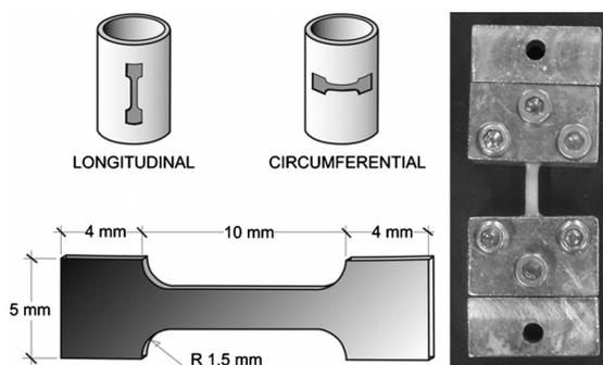
Figure 3: Longitudinally and circumferentially excised aortic sections mounted on a uniaxial testing unit. Adapted from Guinea et al. 2010.
