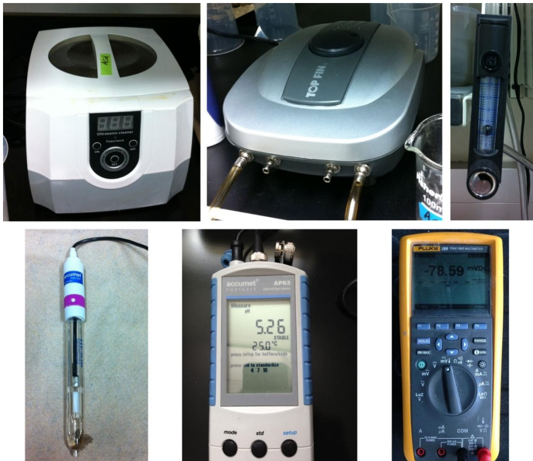
FIGURE 3.2: SHRP test equipment: cleaner, air pump, flow meter, electrode, and meters
