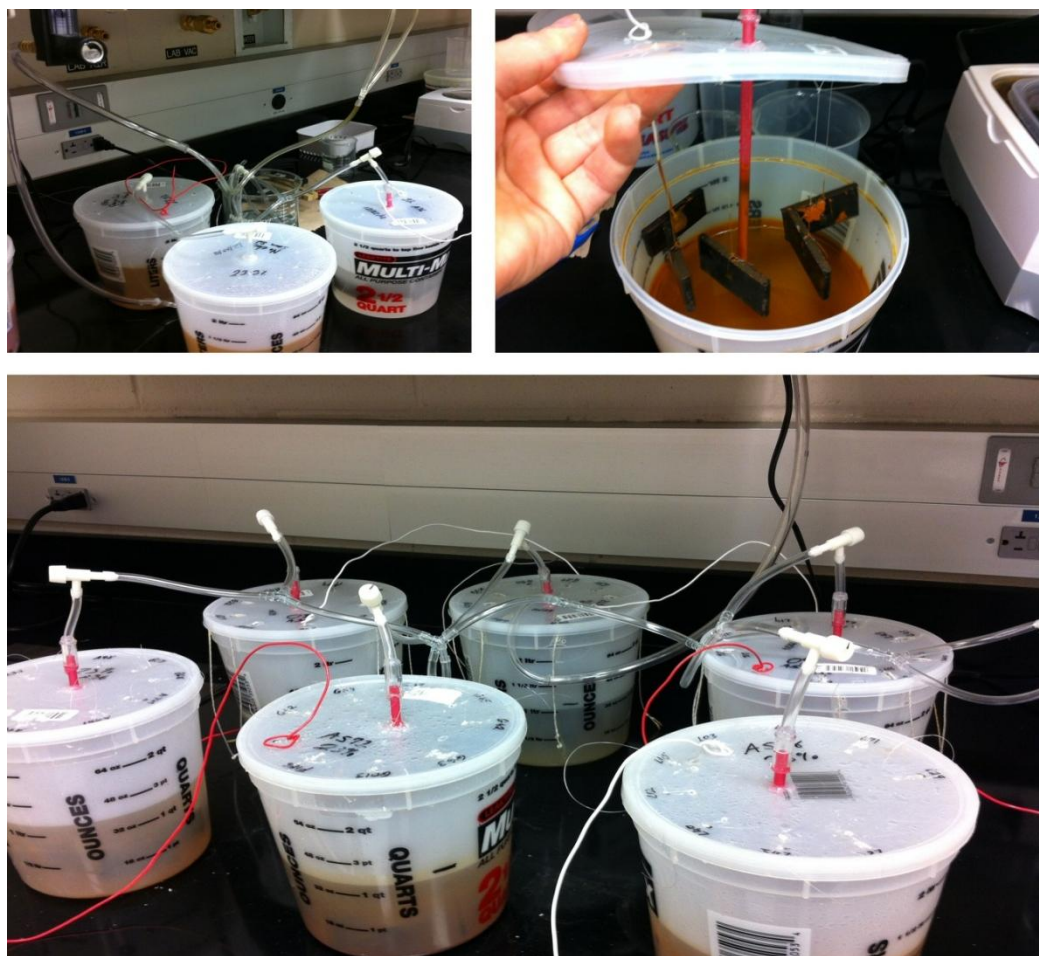
FIGURE 3.3: SHRP H-205.7 test setup with specimens submerged in solution
