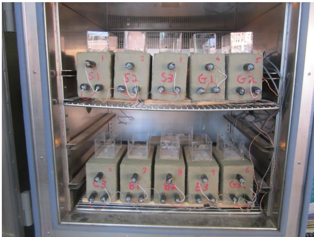
FIGURE 5.5: Finished specimens with attached wires and resistors
