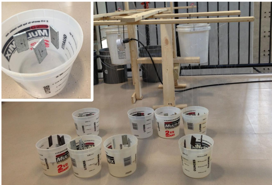
FIGURE 3.20: Scribe test set-up for cyclic wetting and drying corrosive exposure
