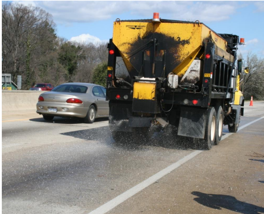
FIGURE 2.1: Granular salt application with auger type spinner
