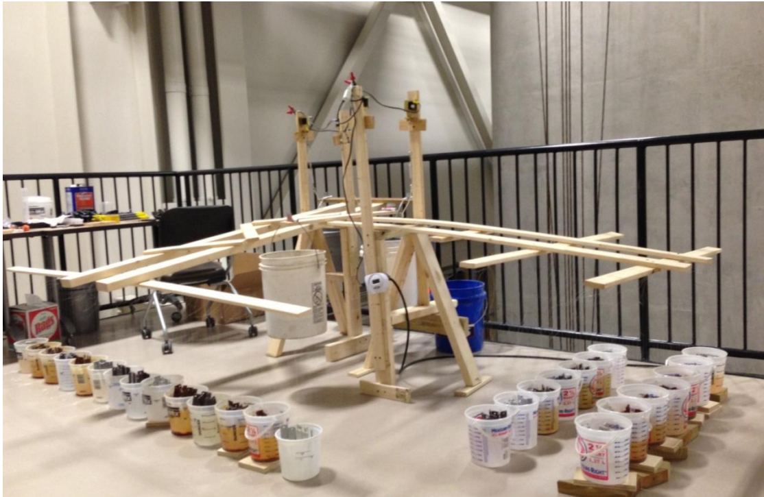
FIGURE 3.9: Fixtures used for dunking motion in cyclic corrosion test
