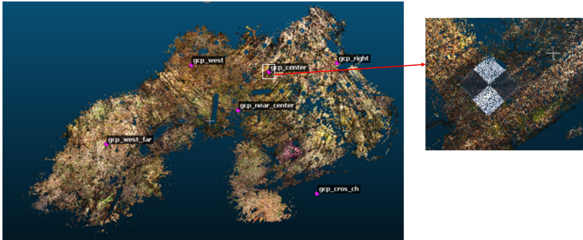
Figure 2.5: Georeferencing the resultant point cloud using 0.61 m X 0.61 m GCP (visible in inset) measured using RTK GPS
