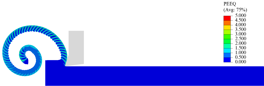
(b) PEEQ results for cutting speed V_c = 400 m/min; \alpha = 17.5^\circ ; a_c = 0.3 mm
