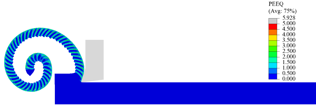
(a) PEEQ results for uncut chip thickness a_c = 0.4 mm; \alpha = 17.5^\circ ; V_c = 400 m/min
