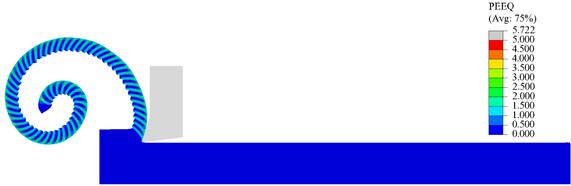
(a) PEEQ results for cutting speed V_c = 800 m/min; \alpha = 17.5^\circ ; a_c = 0.3 mm
