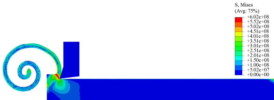
(c) equivalent stress results for rake angle \alpha = 17.5^\circ ; a_c = 0.2 mm; V_c = 800 m/min
