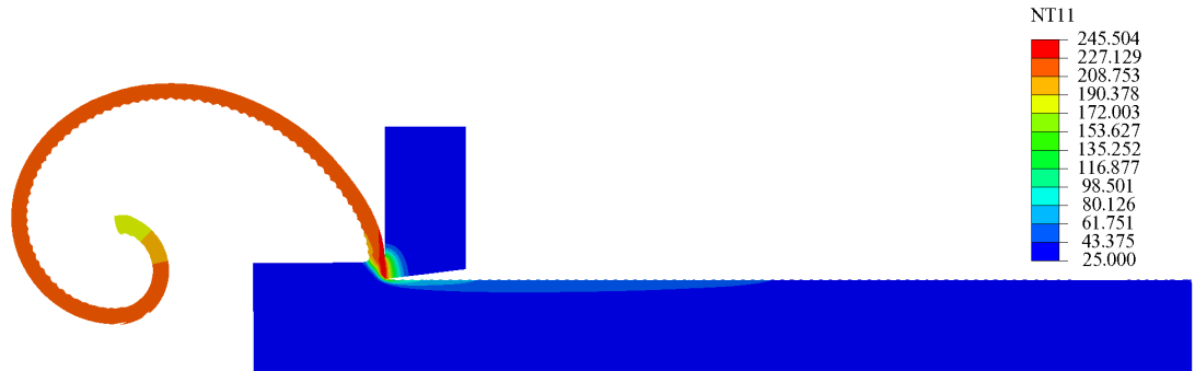
(c) Temperature distribution for uncut chip thickness a_c = 0.2 mm; \alpha = 0^\circ ; V_c = 400 m/min
