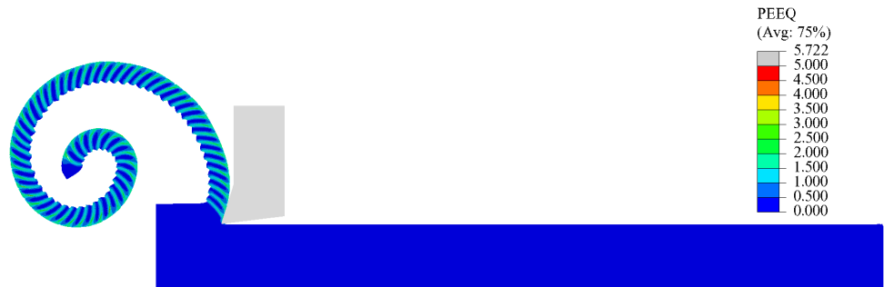
(c) PEEQ results for rake angle \alpha = 17.5^\circ ; a_c = 0.3 mm; V_c = 800 m/min
