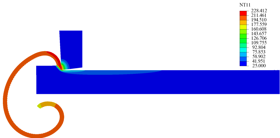
(c) Temperature distribution cutting speed V_c = 200 m/min; \alpha = -3^\circ ; a_c = 0.2 mm
