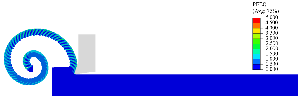
(b) PEEQ results for uncut chip thickness a_c = 0.3 mm; \alpha = 17.5^\circ ; V_c = 400 m/min
