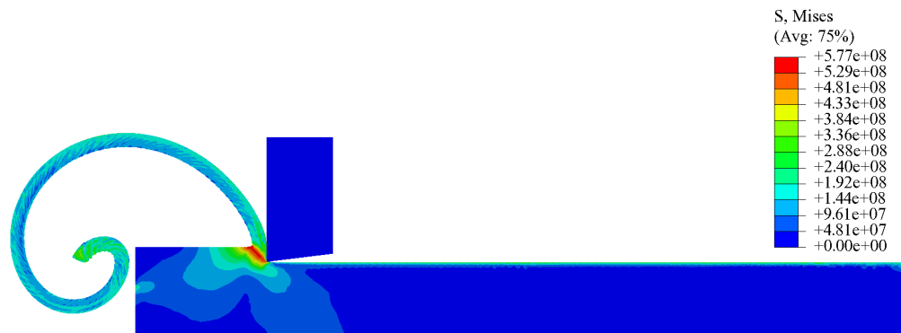
(c) equivalent stress results for uncut chip thickness a_c = 0.2 mm; \alpha = 0^\circ ; V_c = 200 m/min
