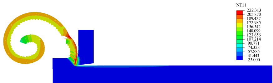
(c) Temperature distribution for rake angle \alpha = 17.5^\circ ; a_c = 0.4 mm; V_c = 800 m/min
