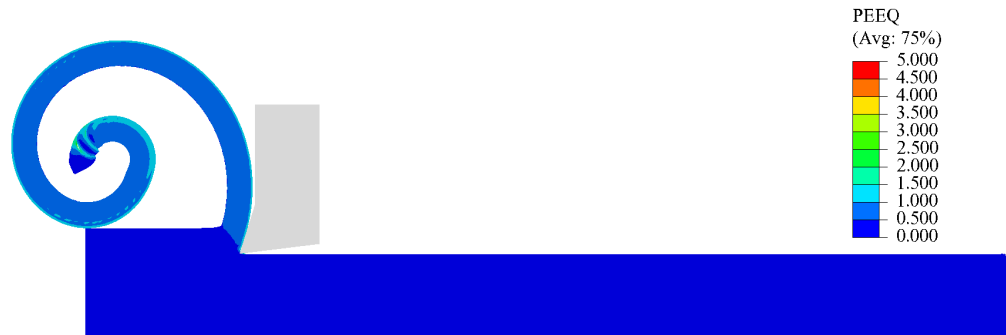
(c) PEEQ results for cutting speed V_c = 200 m/min; \alpha = 17.5^\circ ; a_c = 0.3 mm
