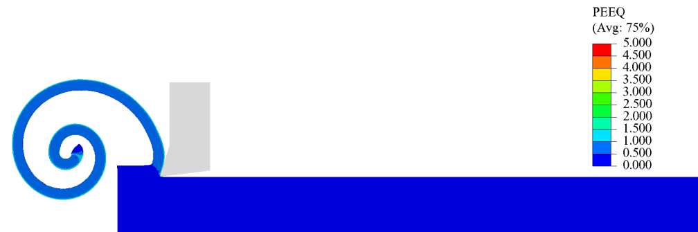
(c) PEEQ results for uncut chip thickness a_c = 0.2 mm; \alpha = 17.5^\circ ; V_c = 400 m/min
