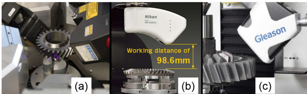
Figure 1.16: Commercial optical measuring instruments: a) MS3D [27] b) Nikon HN-C3030 [28] c) Gleason 300GMSL [29] [after 26]
