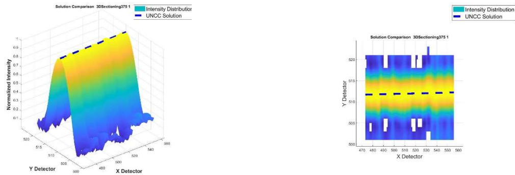
Figure 4.4: Light intensity distribution vs. UNCC solution for a straight ridge line in flat surface measurement
