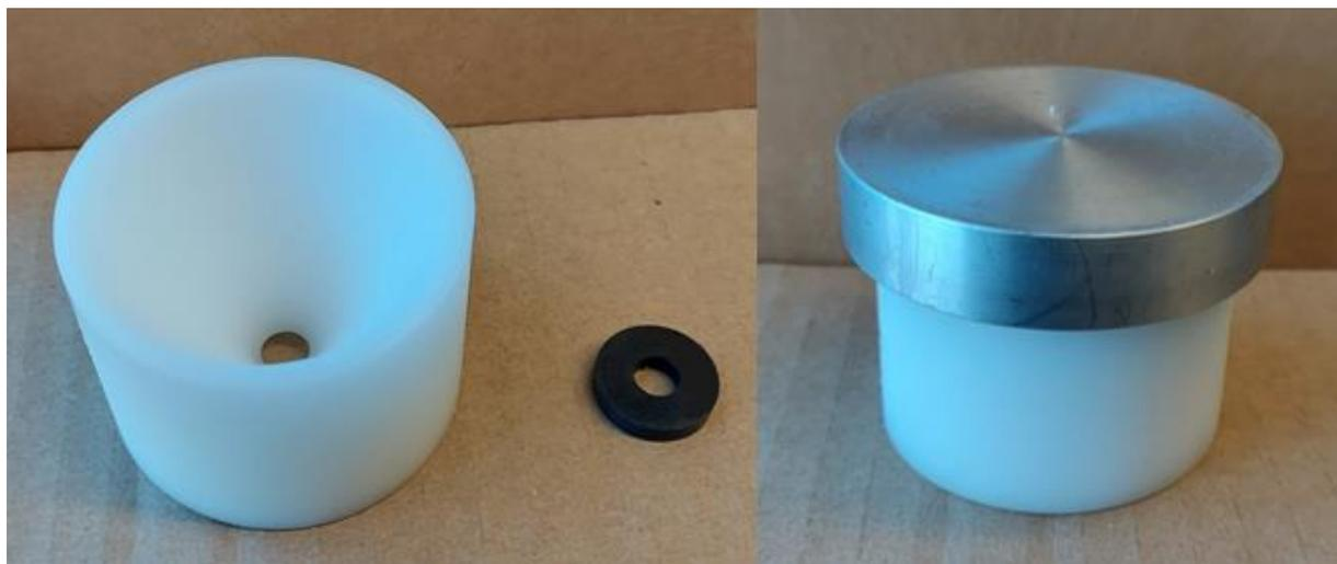
Figure 60 Sample holder ring and cover and sample holder lid machined from acetal and aluminum, respectively.
