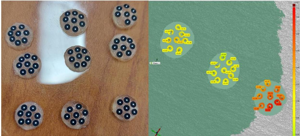
Figure 2 Reference points were used to register the top surface of the alginate-gelatin using the ATOS Scanbox (left). The thickness was estimated as the distance between the surface below the alginate-gelatin and the reference points (right). The thickness of the reference points was removed to define the thickness of the alginate-gelatin alone at each point.
