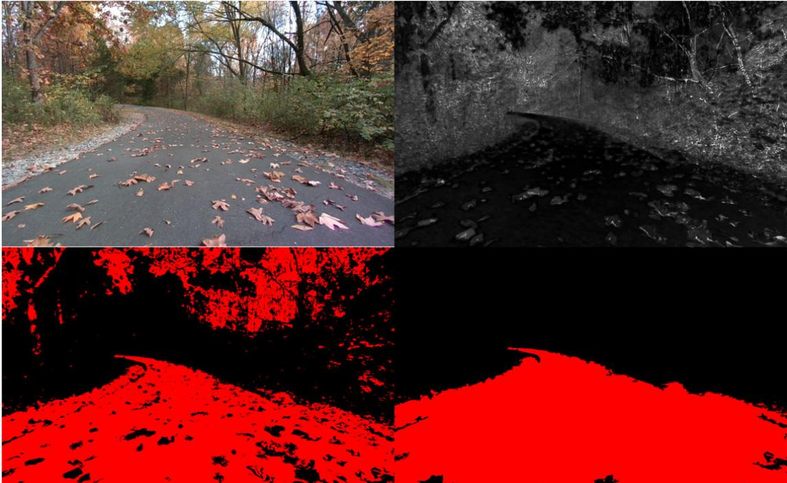
Figure 31: Binary Path Detection: Upper Left (UL): Color Image, Upper Right (UR): Saturation Plane. Lower Left (LL): Binary Threshold, Lower Right (LR): Advanced Morphology
