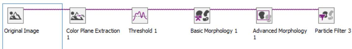
Figure 102: Asphalt Detection Script
