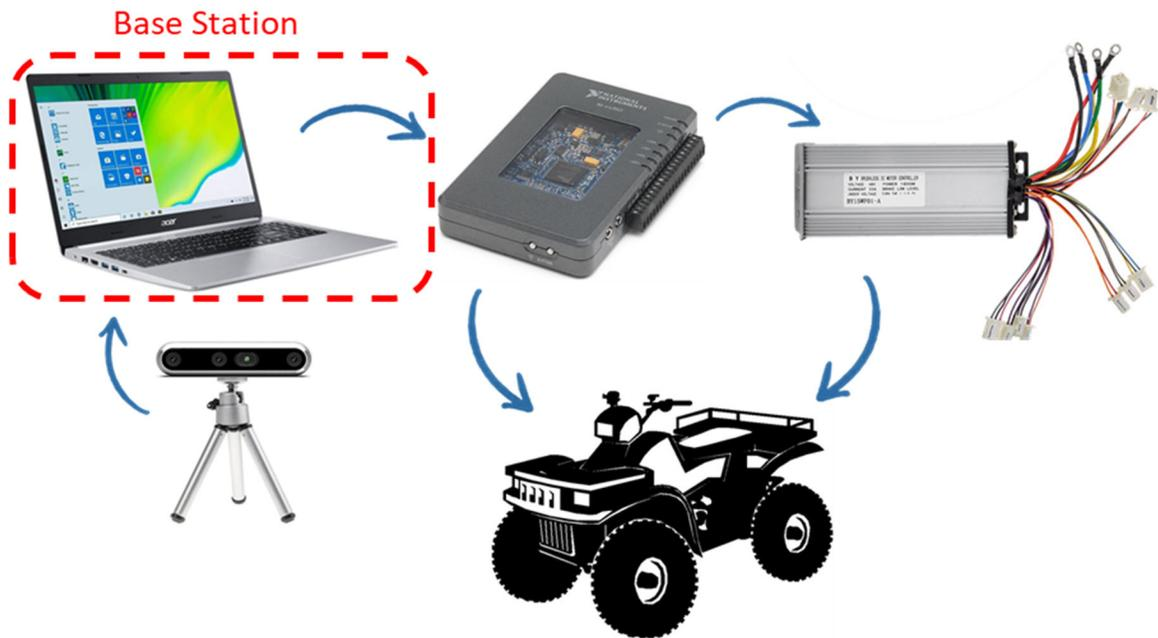
Figure 29: Hardware Configuration for Autonomous Vehicle Control
