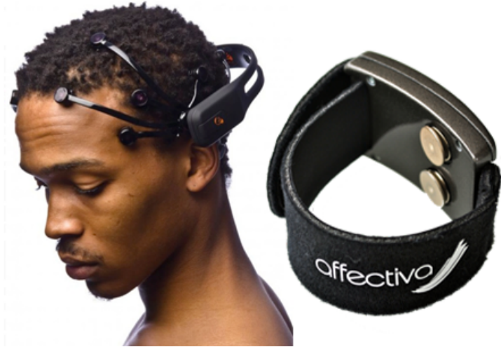
Figure 12: The Emotiv EEG headset (left) and Affectiva Q sensor (right) were used in the ITMC study to capture physiological responses. The Emotiv headset is a wireless EEG device, and the Q includes EDA, skin temperature, and a 3-axis accelerometer.
