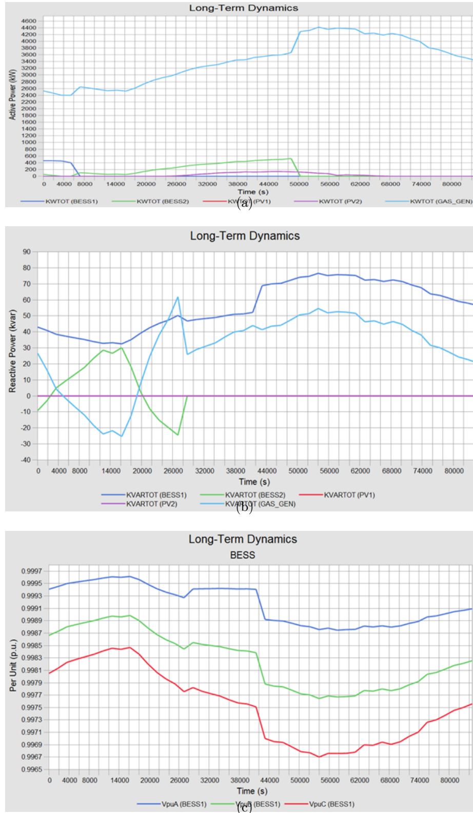
Figure 4.9: BESS2 Possible Location 1 (a) Active Power of different resources , (b) Reactive Power of different resources, (c) voltage profiles at BESS POI .
