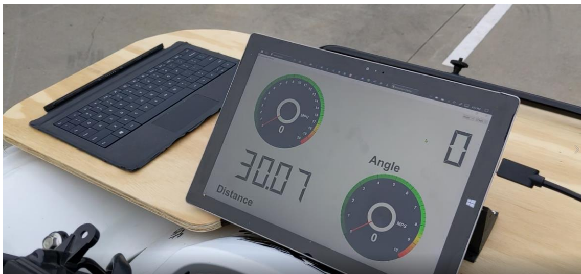
FIGURE 4.19: Odometry results from 30-meter measured drive
