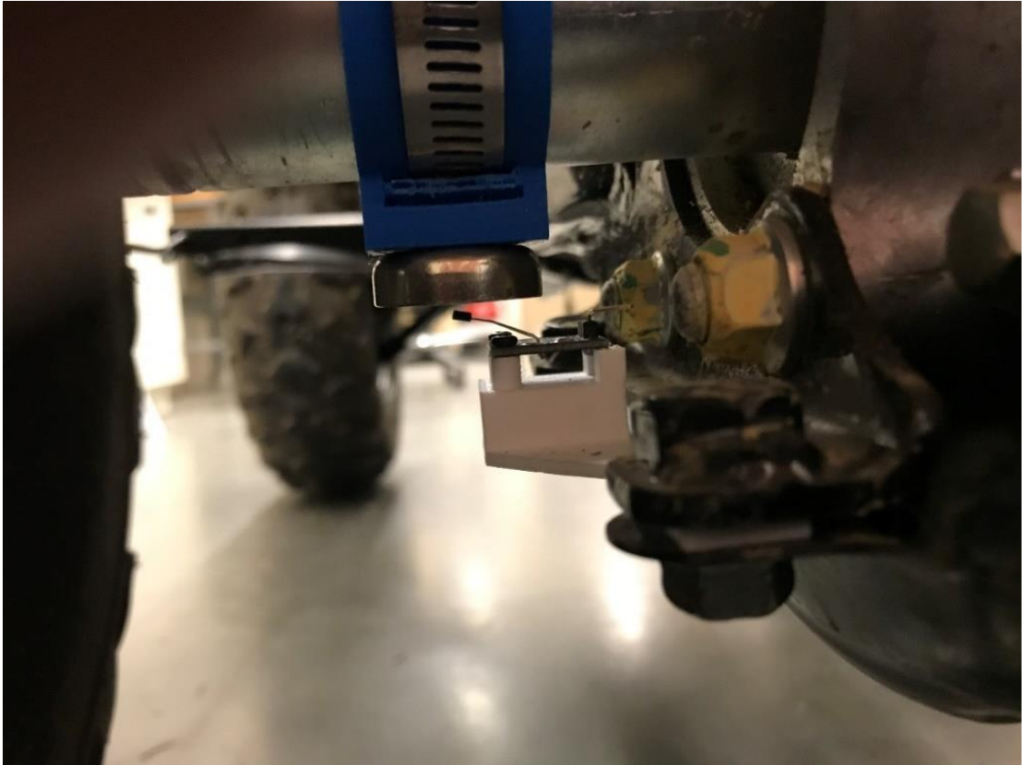
FIGURE 4.11: Distance clearance of encoder and Hall effect sensor
