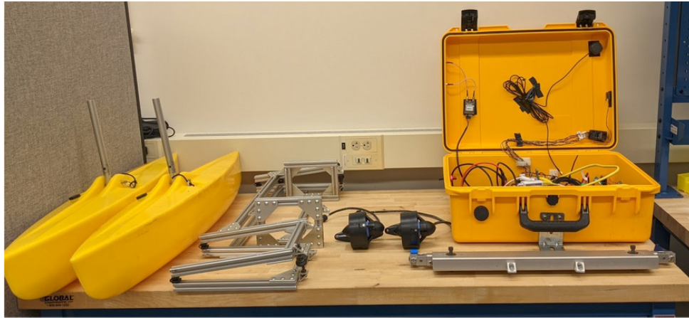
Figure 5.8: Deconstructed ASV for transport and storage.
