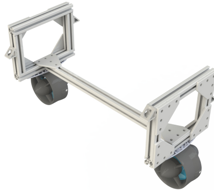
Figure 5.9: ASV propulsion system and framing.
