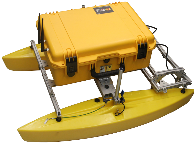
Figure 5.10: Final ASV build excluding sensor package.
