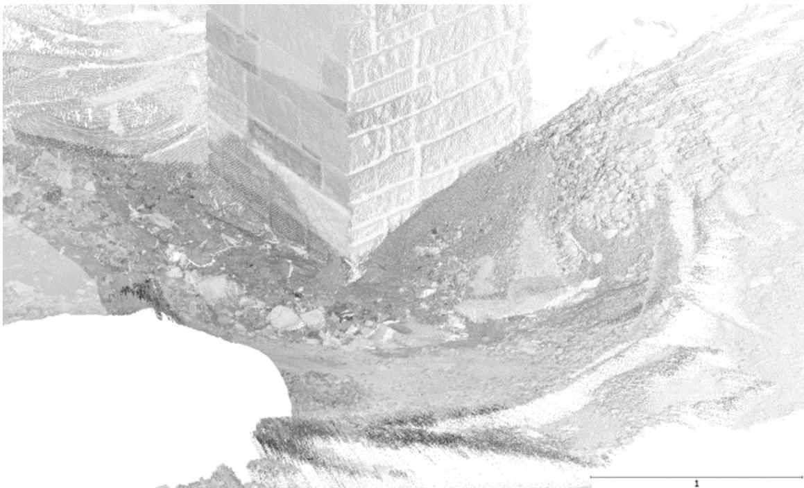
Figure B-3 Point cloud of Phillips Road Bridge North Bank Pier No. 2 and scour as on June 9, 2020
