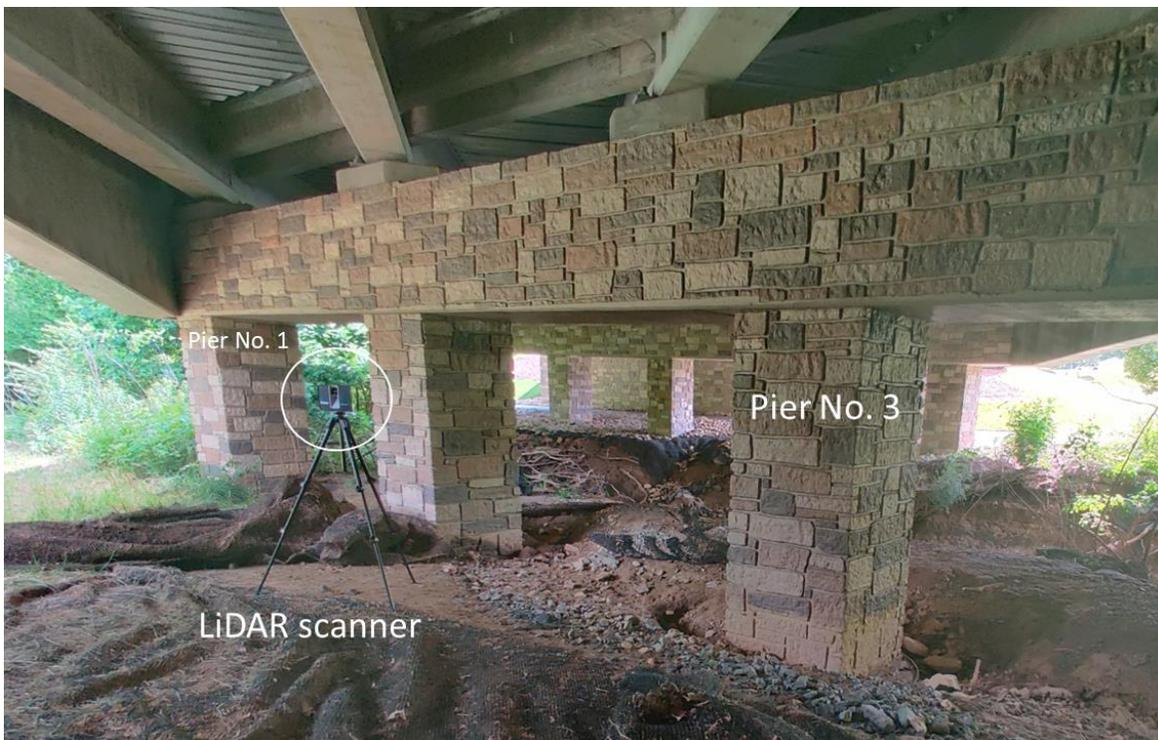
Figure A-4 LiDAR scan in progress (June 9, 2020)
