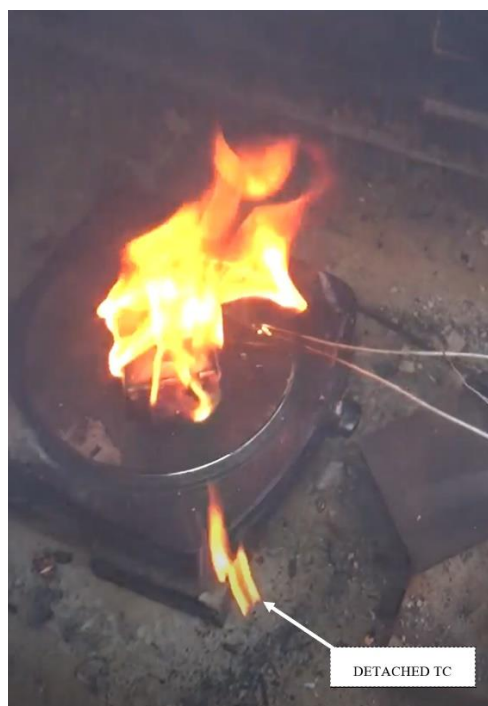
Figure 5-17: Top-cell DAQ TC detaching [7:31 (vid.), 417sec (data)] 6.8.22
