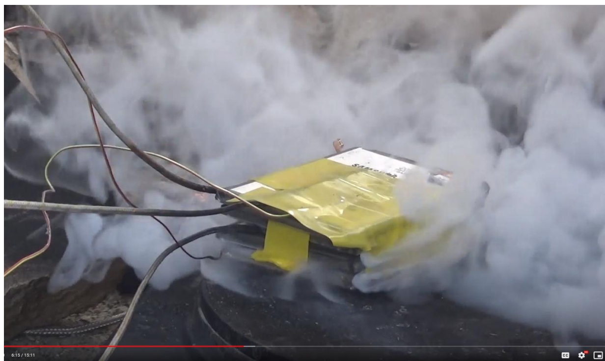
Figure 5-27: ~5sec into first hiss/smoke (bottom cell) [6:15 (vid.), 335sec (data)] 6.11.22
