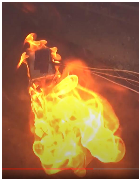
Figure 5-9: First jet after 2sec, bottom cell, [7:13 (vid.), 399sec (data)] 6.8.22
