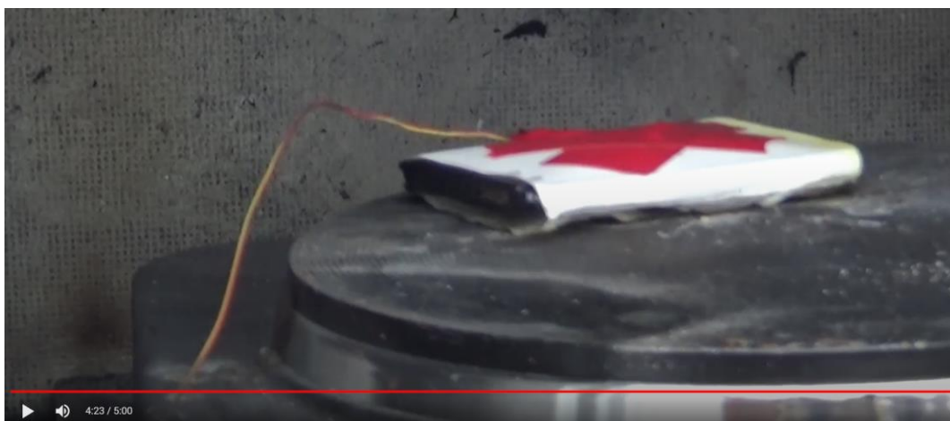
Figure 4-2: 1sec before rapid expansion/explosion [4:23 (vid.), 245sec (data)] 5.4.22
