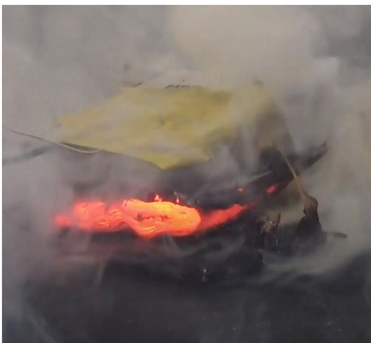
Figure 5-32: Red-hot innards after hiss/expans. (2 nd cell) [9:38 (vid.), 538sec (data)] 6.11.22
