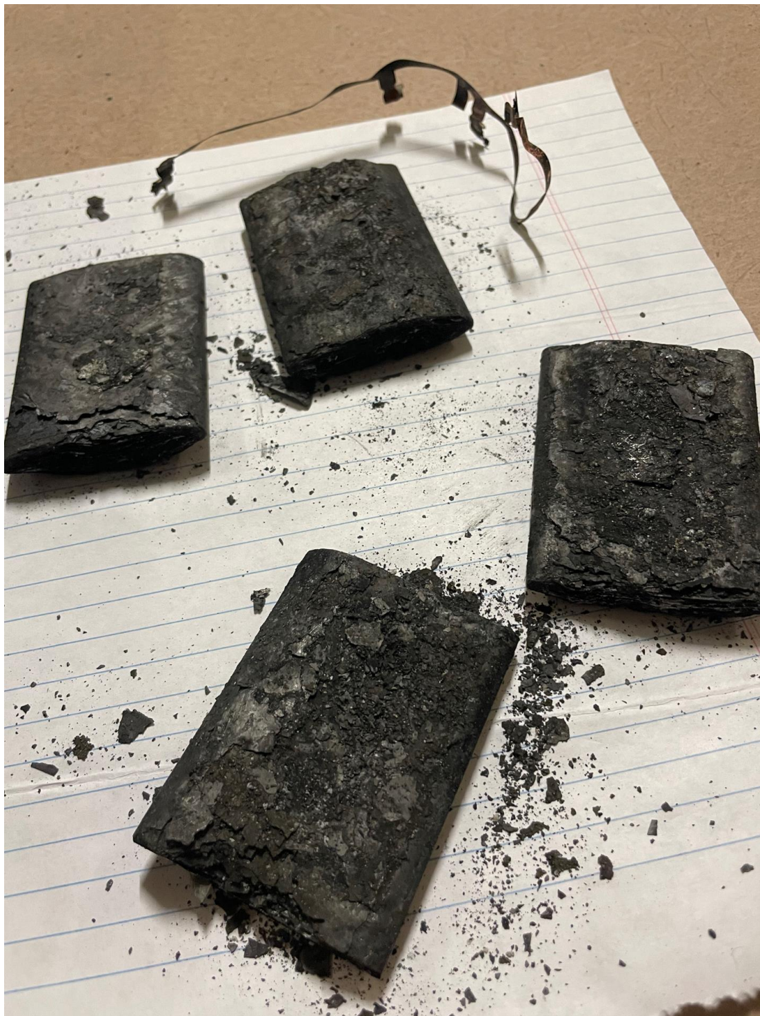
Figure 5-25: Post-condition of all 4 cells (order unknown) 6.8.22
