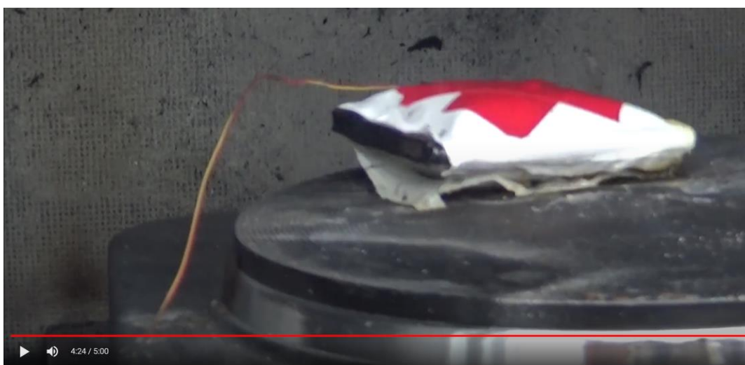
Figure 4-3: Maximum expansion before explosion [4:24 (vid.), 246sec (data)] 5.4.22
