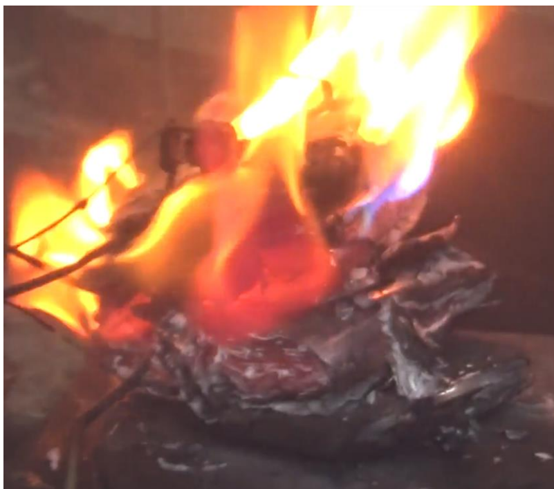
Figure 5-40: After jets, partially blue flame (3 rd cell) [10:25 (vid.), 585sec (data)] 6.11.22
