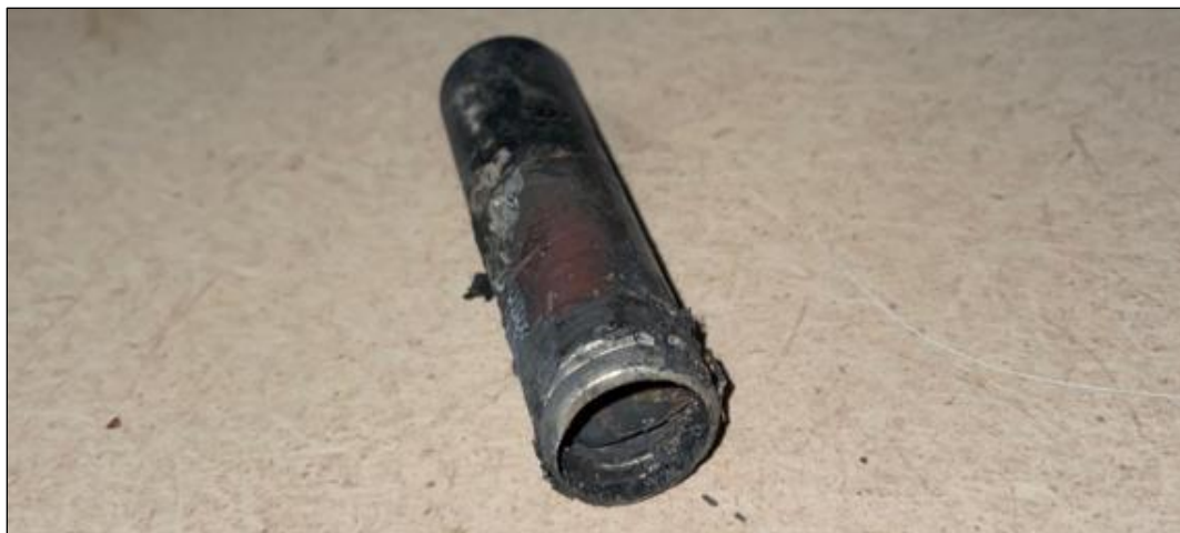
Figure 5-70: Post-condition photo, emptied bottom cell, 6.11.22(18650)
