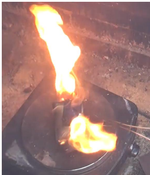
Figure 5-19: 3 rd and final jets both sides, (top cell only?) [7:40 (vid.), 426sec (data)] 6.8.22
