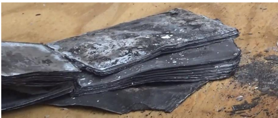
Figure 5-47: Hot internal cell layers, flipped open (cell unknown) 6.11.22
