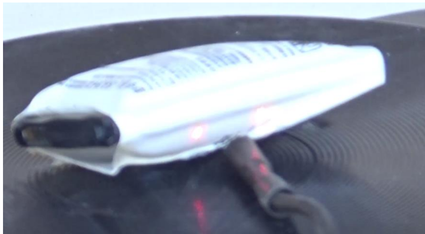
Figure 6-2: Phase 2, medium expansion, ICR 3.2.22
