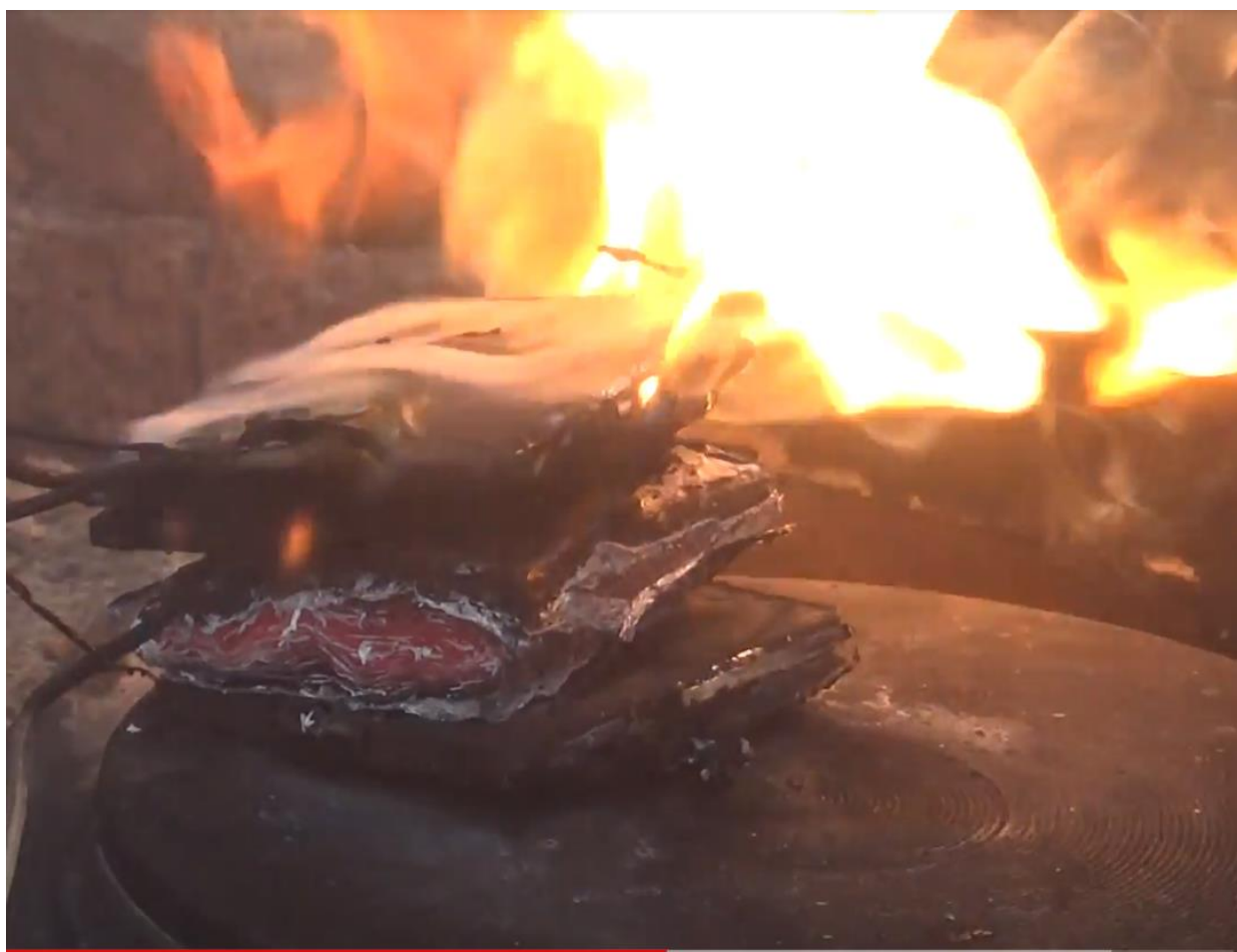
Figure 5-36: 3 rd hiss w/ instant jet flames (3 rd cell) [10:13 (vid.), 573sec (data)] 6.11.22
