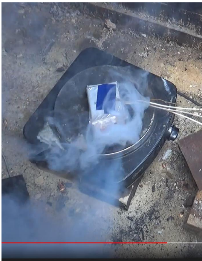
Figure 5-4: First hiss after 1sec, bottom cell [6:59 (vid.), 384sec (data)] 6.8.22
