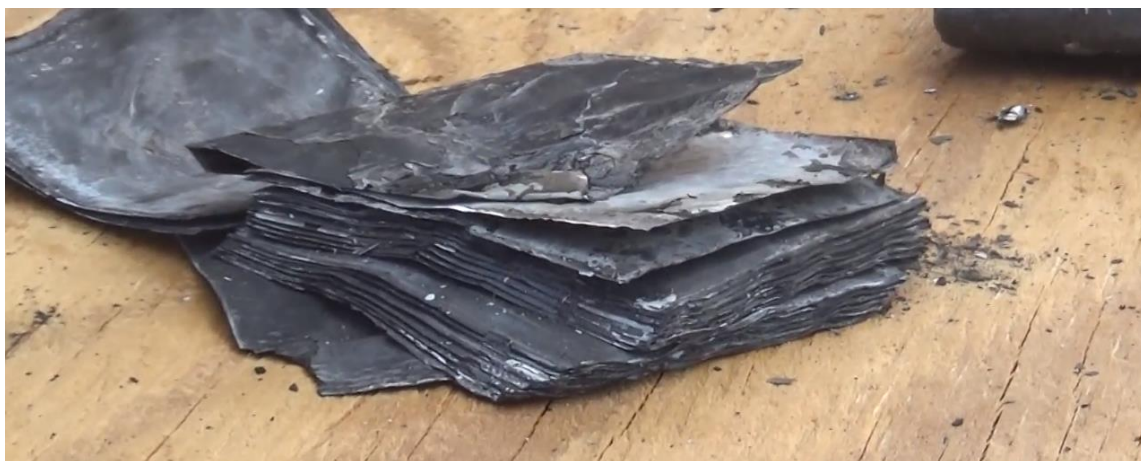
Figure 5-46: Hot internal cell layers (cell unknown) 6.11.22
