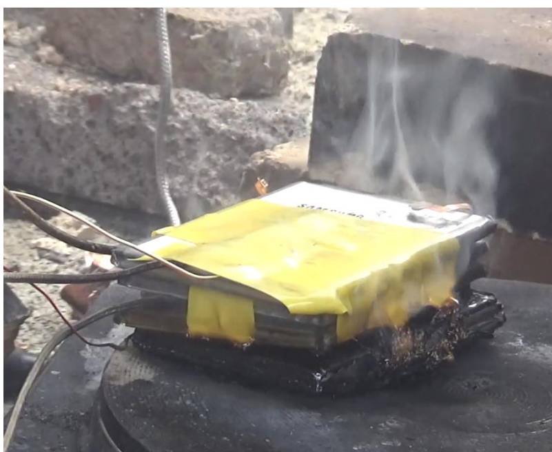
Figure 5-29: Bottom cell post-hiss condition, no fire [7:44 (vid.), 424sec (data)] 6.11.22
