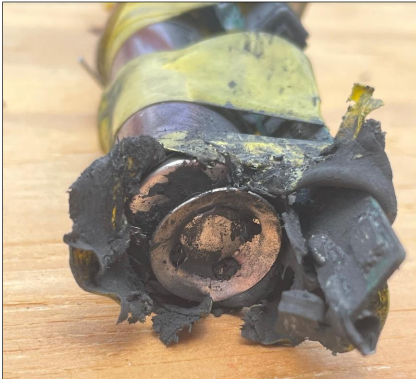
Figure 5-69: Post-condition photo, implanted (+) end cap, 6.11.22(18650)
