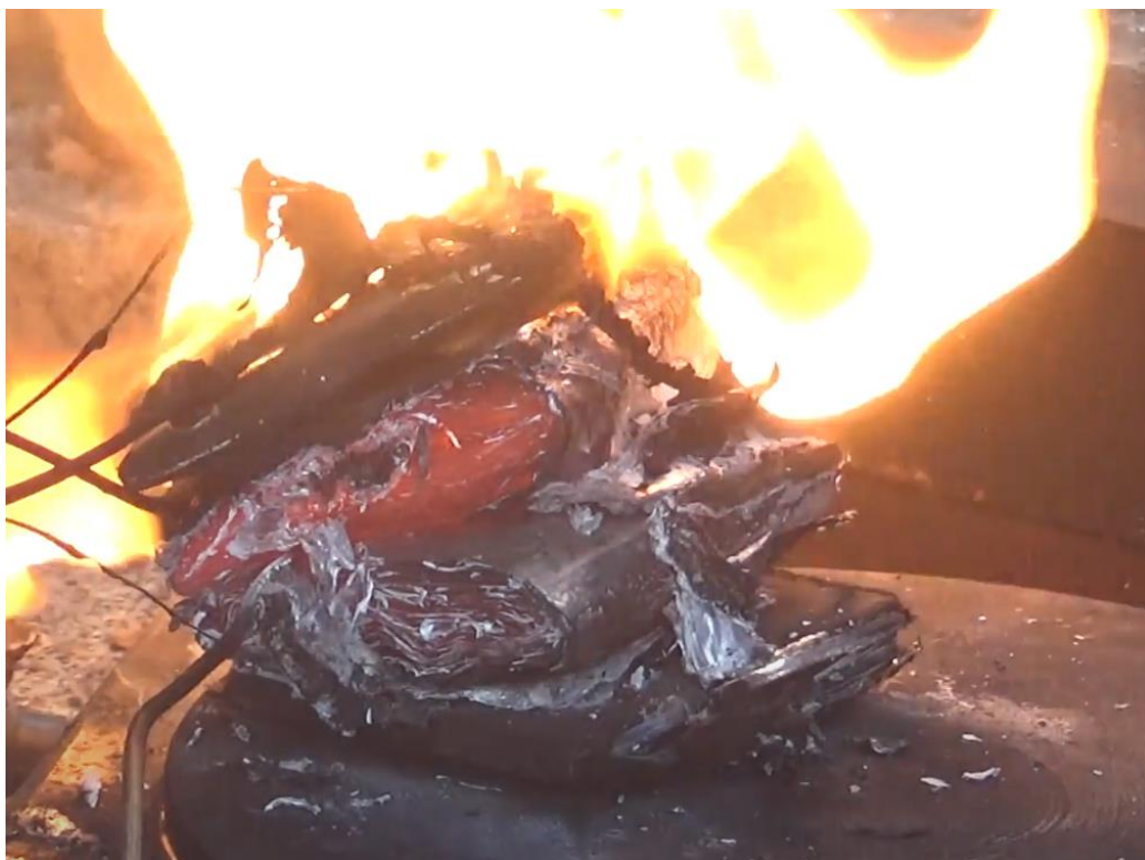
Figure 5-42: Start of jet flames before falling (4 th cell) [10:44 (vid.), 604sec (data)] 6.11.22
