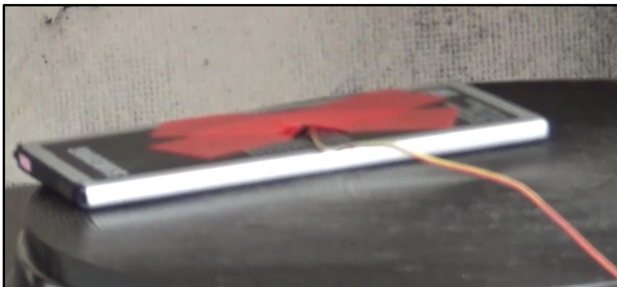
Figure 3-8: Single prismatic cell placement
