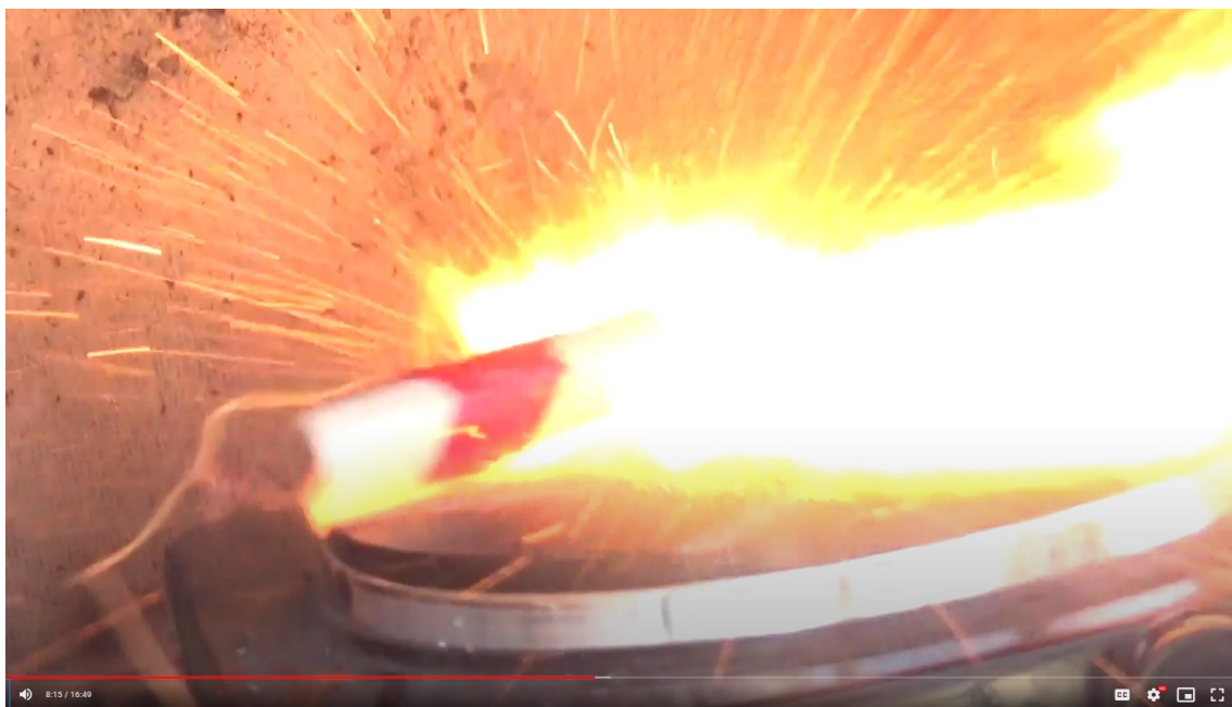
Figure 4-11: Moment of explosion [8:15 (vid.), 399sec (data)]4.27.22 (3)
