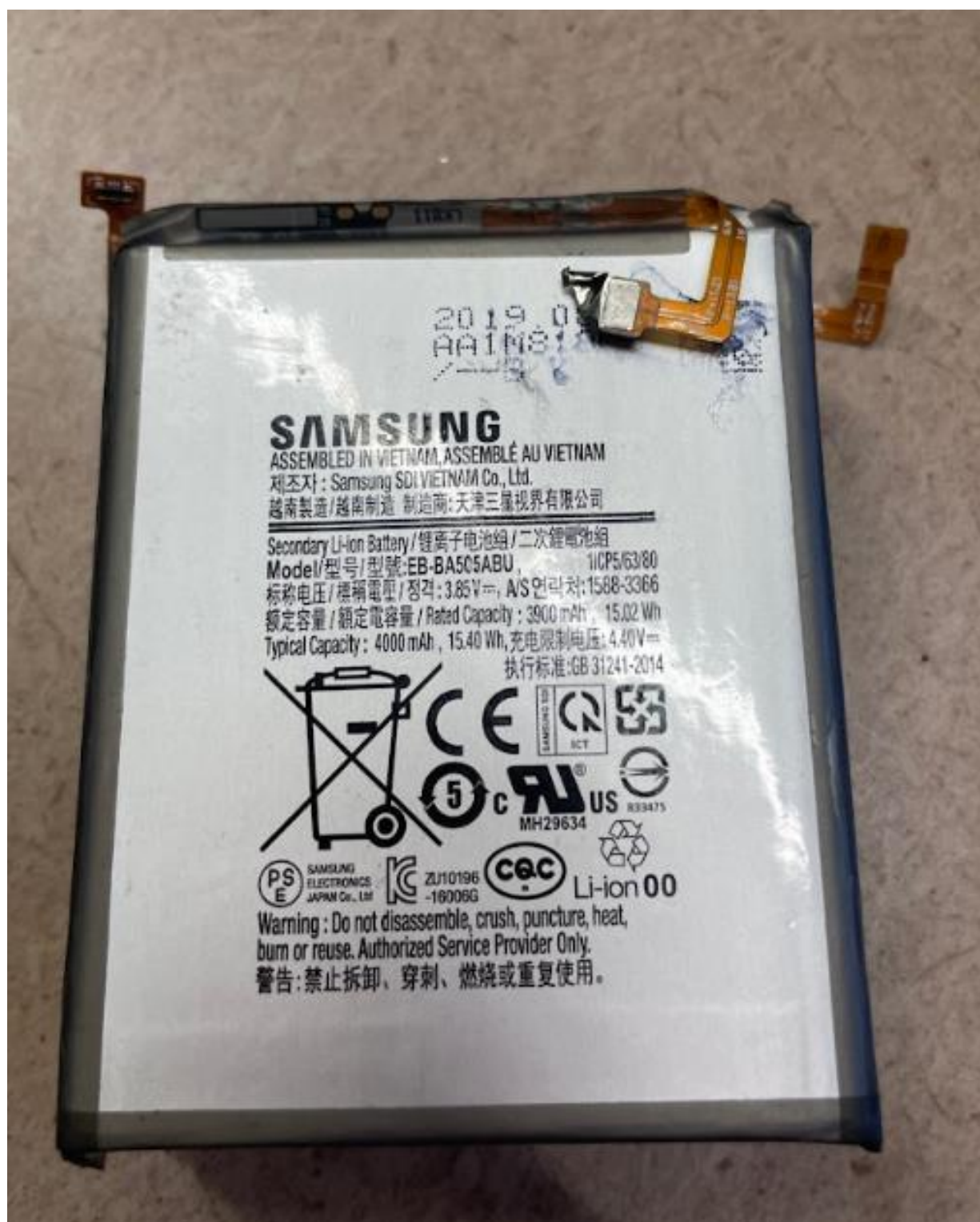
Figure 5-2: Label of multi-pouch test cells
