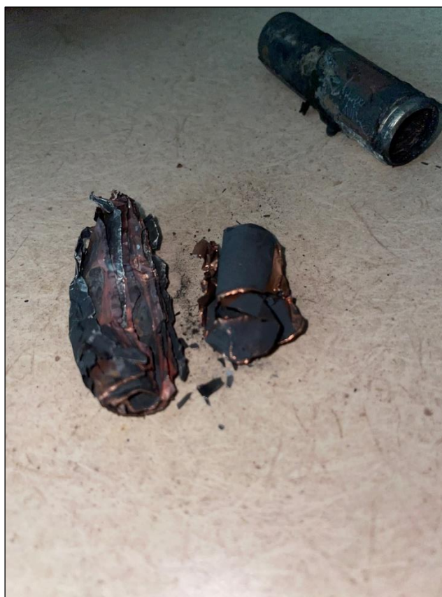
Figure 5-71: Post-condition photo, bottom cell w/ ejected innards, 6.11.22(18650)
