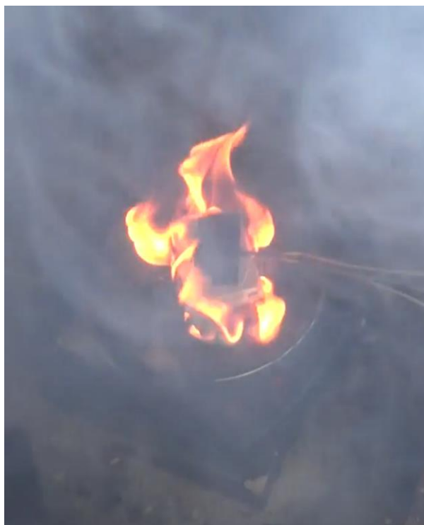
Figure 5-7: First ignition, bottom cell [7:05 (vid.), 391sec (data)] 6.8.22
