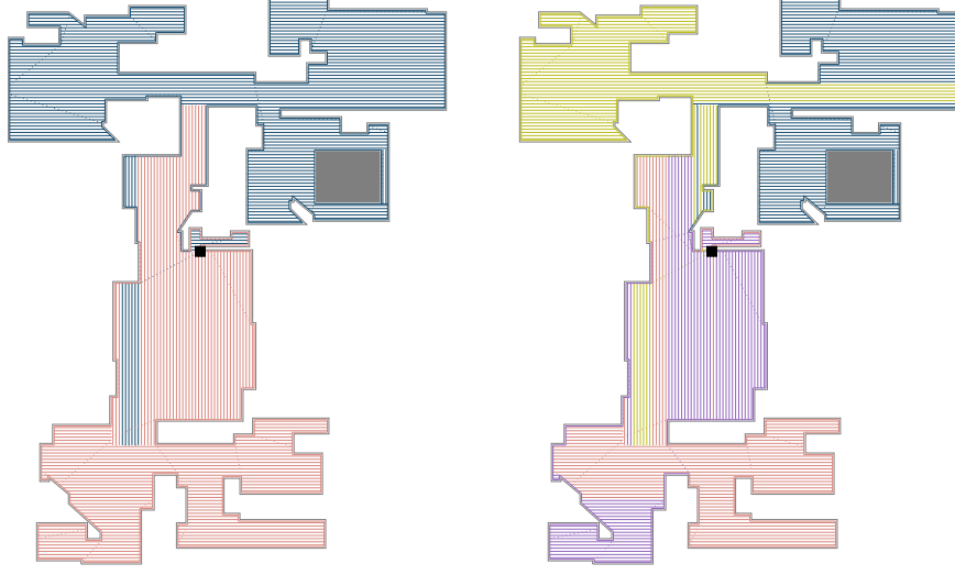
Figure 4.4: Coverage of a large indoor environment with 107 \text{ m}^2 area and 151 vertices, given in Vandermeulen et al. (2019). The left figure shows our solution for two robots with a tool width of 0.1 \text{ m} and a capacity of 700 \text{ m} , with tour costs 616 \text{ m} and 620 \text{ m} . The right figure shows our solution for four robots with a capacity of 320 \text{ m} , with tour costs 312 \text{ m} , 313 \text{ m} , 318 \text{ m} , and 300 \text{ m} .
