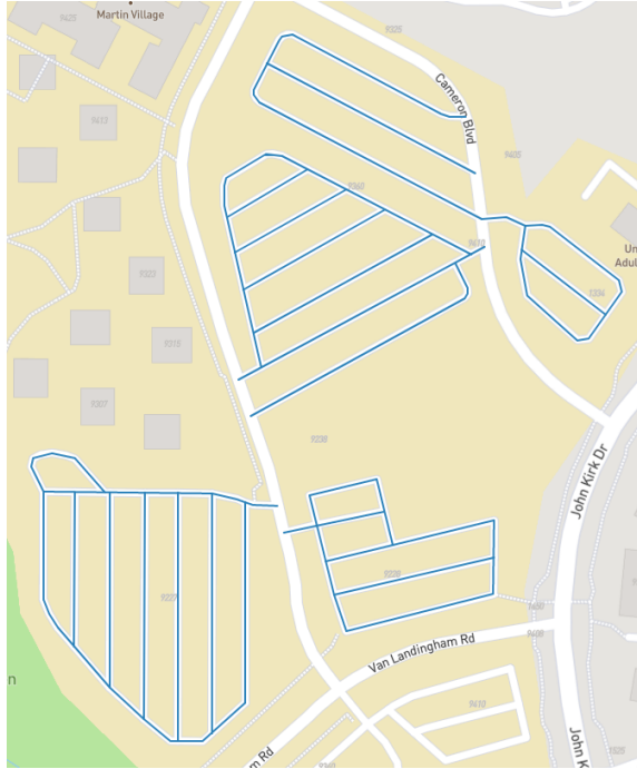
Figure 2.14: A network of lanes specified on a set of parking lots: The total length of the lanes is 2,982 m. There are 90 vertices, 104 required edges, and 4,005 non-required edges. The required edges form four connected components.
