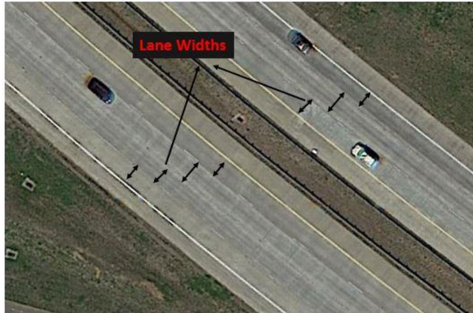
Figure 3 Capturing Lane Widths Using Google Earth Pro Software
