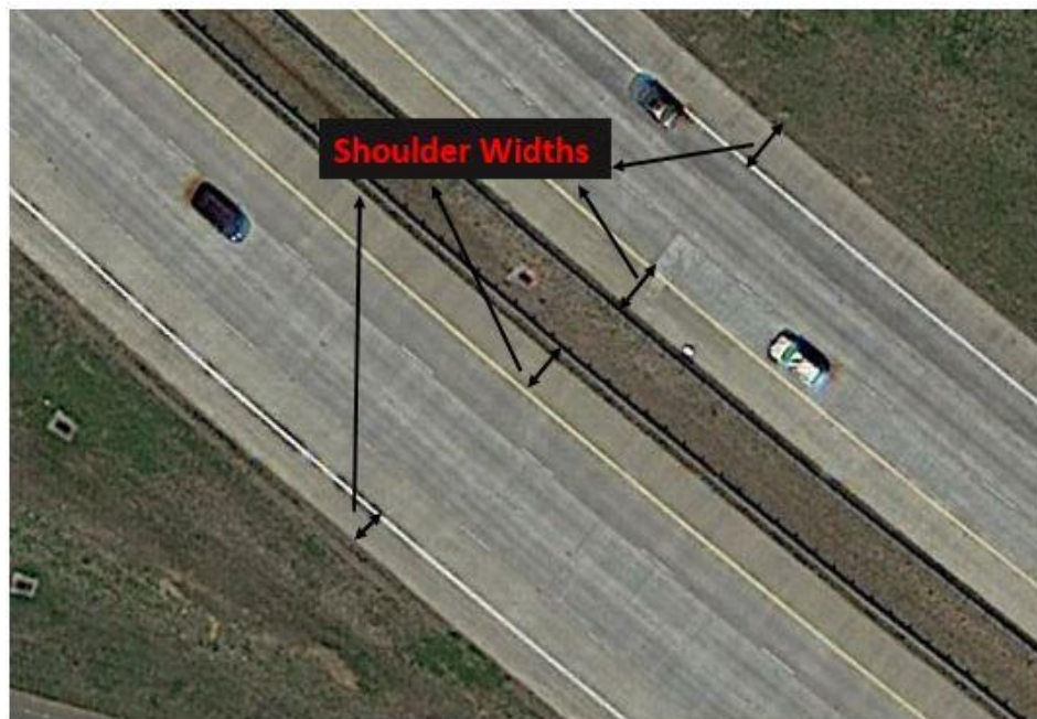
Figure 4 Capturing Shoulder Widths Using Google Earth Pro
