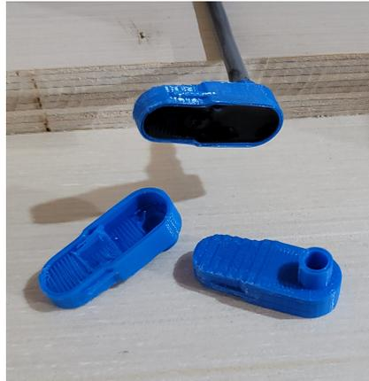
Figure 5.4: Sensor housing with potted sensor electronics.
