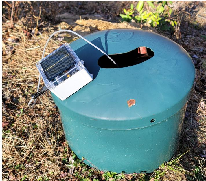
Figure 6.6: Working prototype attached with magnetic feet to an in-ground, 500 gallon tank.
