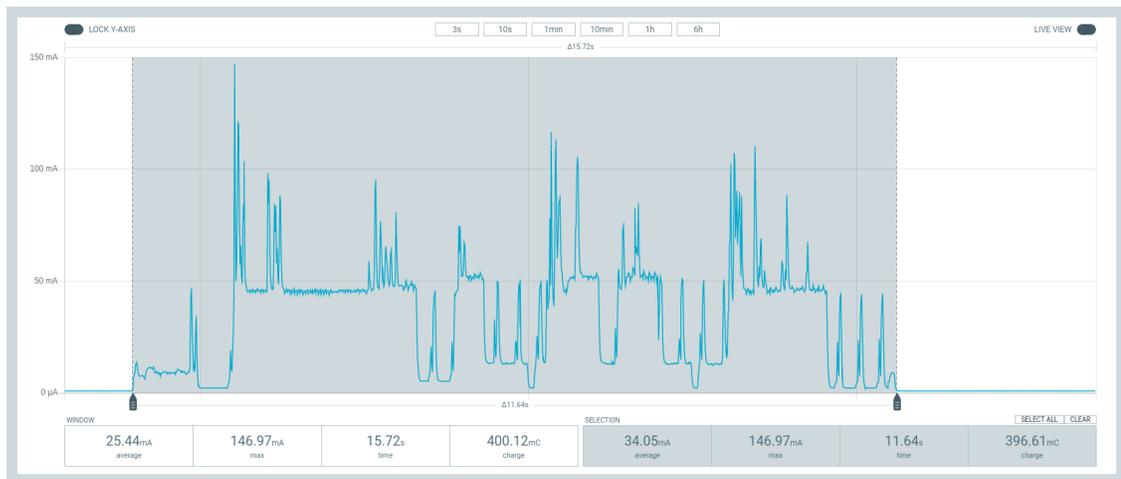
Figure 6.4: Power profile window during a cellular transmission cycle at -126 dBm.
