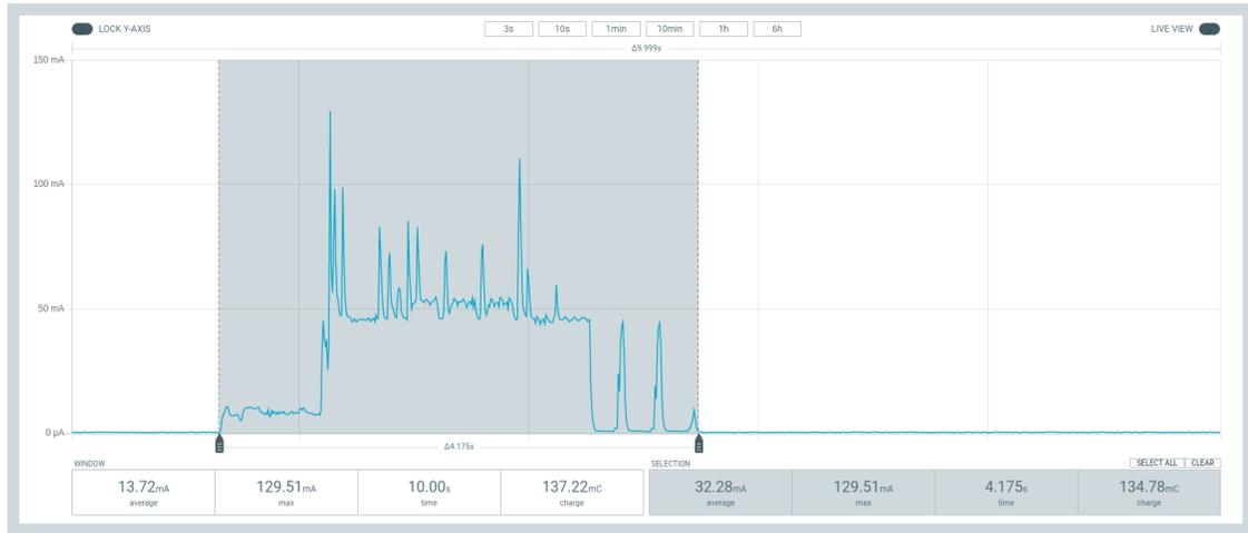
Figure 6.3: Power profile window during a cellular transmission cycle at -105 dBm.
