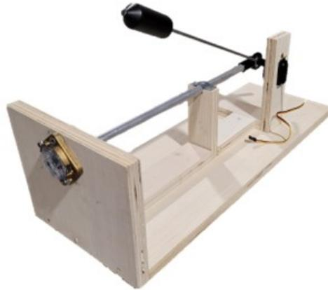
Figure 5.5: Tank level testing jig with servo positioning.
