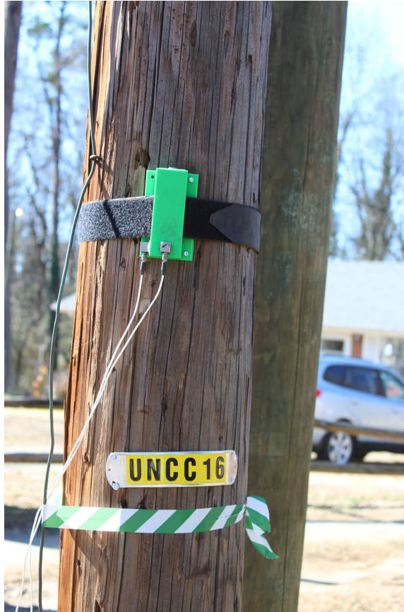
FIGURE 1.4: Prototype and wired accelerometers secured to pole Pole 16 on Axis 1 at an elevation of 6 feet above ground
