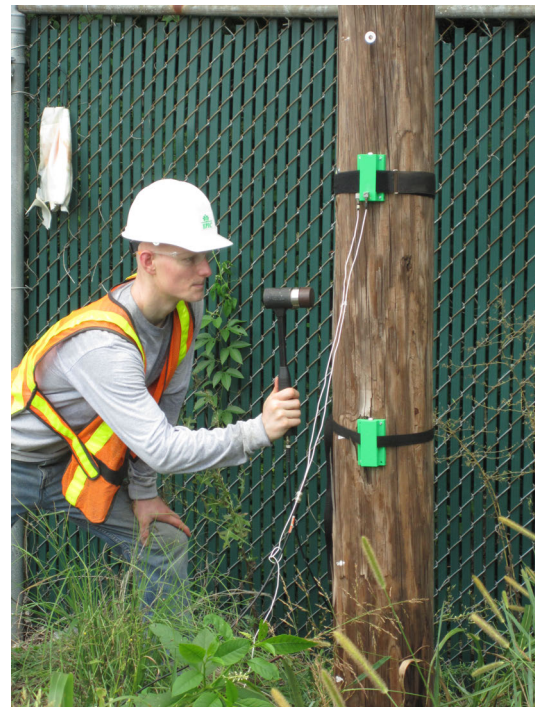
FIGURE 5.6: Impulse excitation of modes in direction of axis 2 at a) 6 feet b) 4 feet above ground
