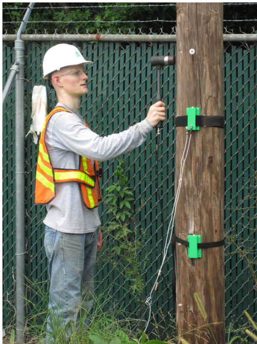
FIGURE 5.6: Impulse excitation of modes in direction of axis 2 at a) 6 feet b) 4 feet above ground
