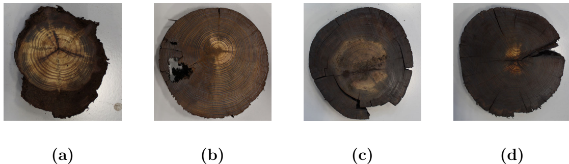
FIGURE 1.1: Common types of cross section damage: (a) shell rot (b) pocket rot (c) shake (d) checking; heart rot not pictured
