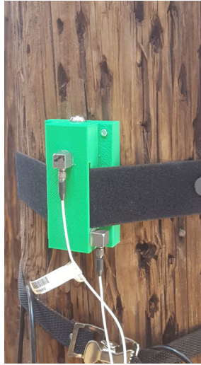
FIGURE 3.15: Photograph of prototype installation on timber pole with cable-based accelerometers installed on the case of prototype for reference measurement
