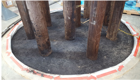
FIGURE 4.20: Asphalt encasement of the second set of ten poles in the experimental test pit
