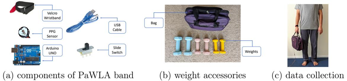
Figure 6.1: PaWLA prototype and data collection: (a) hardware components of PaWLA Band; (b) weight accessories; (c) data collection with a PaWLA band.
