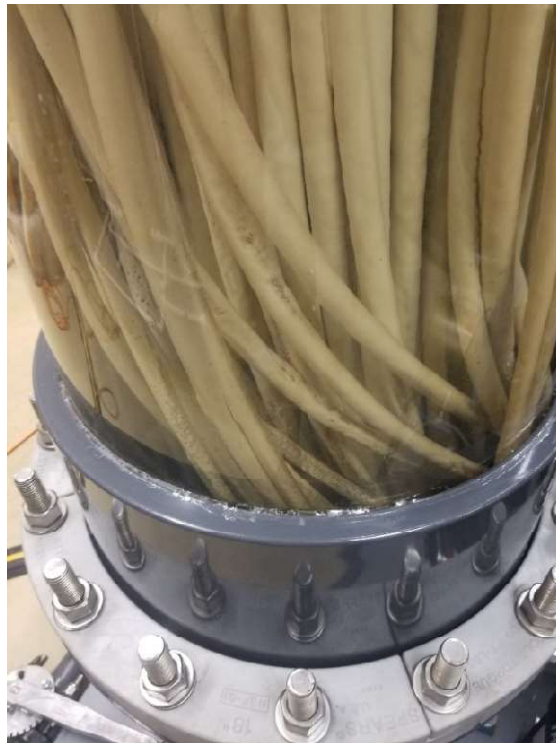
Figure 4.11: Filter elements after 1-hour of filtration at 2.0 \frac{\text{gpm}}{\text{ft}^2}
