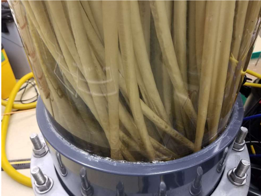
Figure 4.10: Filter elements after 1-hour of filtration at 1.6 \frac{\text{gpm}}{\text{ft}^2}
