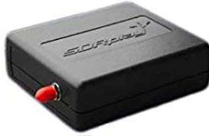
FIGURE 3.5: SDR used – SDRPlay RSP1A[31].
