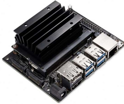
FIGURE 3.6: NVIDIA Jetson Nano 4GB developer kit[26].
