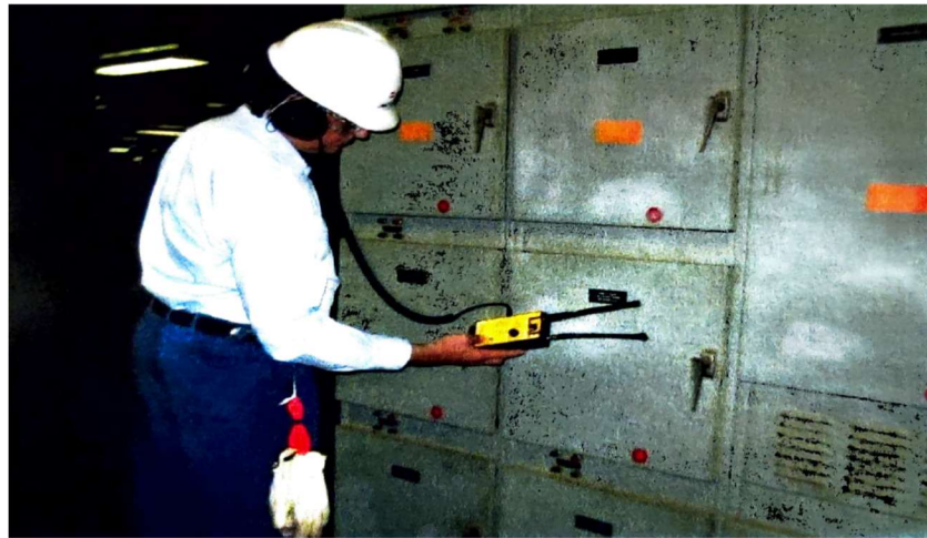
FIGURE 1.2: Engineer using a handheld EMI sniffer to scan switchgear[14].
