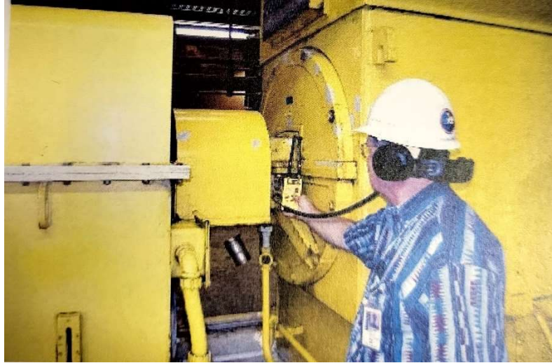
FIGURE 1.1: Engineer using a handheld EMI sniffer to scan motor to receive AM signals[14].
