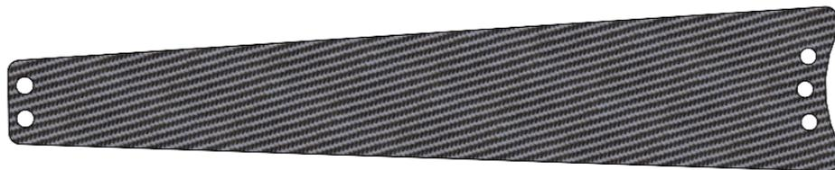
Figure 4.8: Carbon fiber support CAD model for turbine blades
