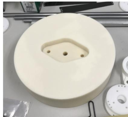
Figure 4.12: Physical 3D printed surrogate generator subassembly of prototype system
