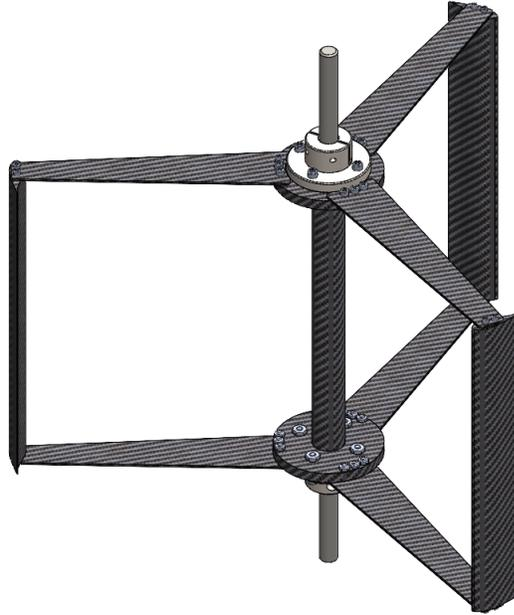
Figure 4.5: CAD model of turbine subassembly of prototype system
