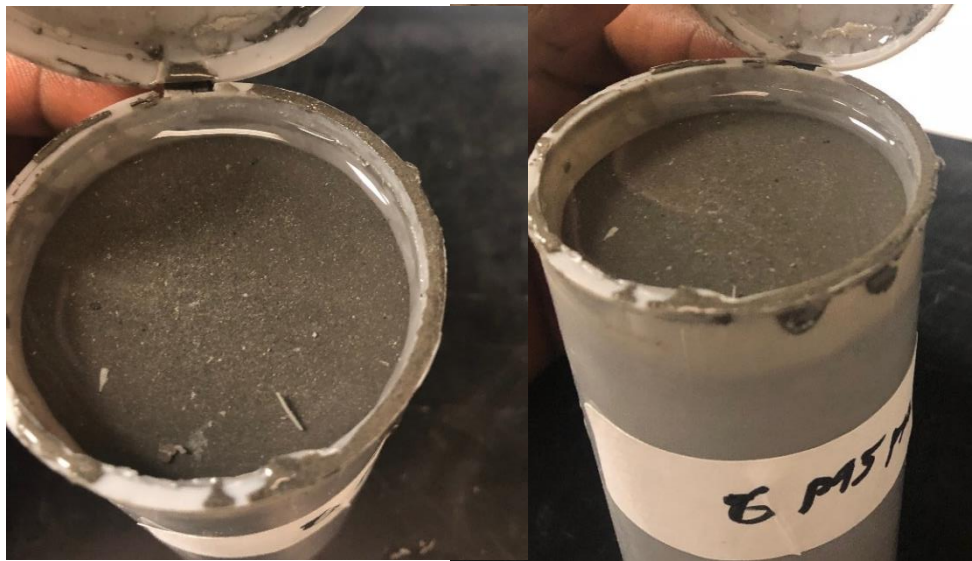
Figure A33: P95FA with bleeding water at 28 days.
